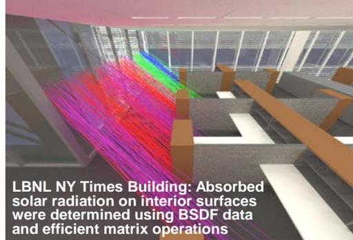
LBNL NY Times Building: Absorbed solar radiation on interior surfaces were determined using BSDF data and efficient matrix operations
