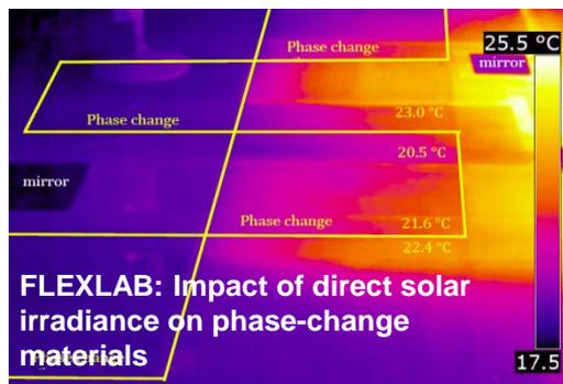
FLEXLAB: Impact of direct solar irradiance on phase-change materials
