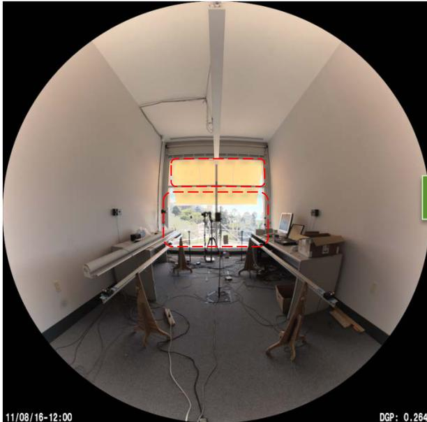
F-matrices for horizontally subdivided window yields good agreement between simulated and measured data for sensors both near and far from the window
