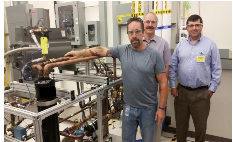
Compressor Calorimeter Test Rig (Phase 1 approved)
