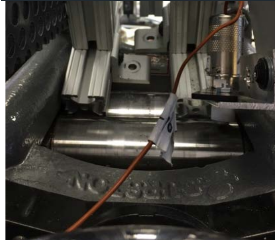
Rolling thermocouple and IR camera used to measure temperatures of moving ribbons
