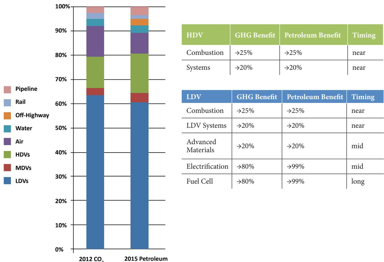
Improved LDV and HDV systems have the potential for significant reductions in transportation petroleum use and GHG emissions. These figures are aggregated from the technology sections. Each estimate is calculated as the per-vehicle impacts times the total opportunity for the affected mode(s). This is intended only as a reference point and not a goal or forecast. Estimates cannot be combined directly with other impact potentials in this chapter due to double counting. (Source: DOE)
