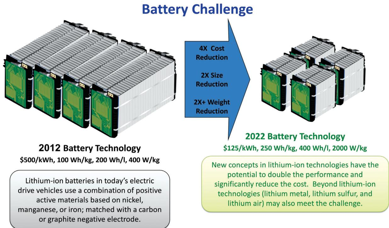
**Figure 8.11** Modeled Cost and Energy Density of PEV Batteries Developed and Tested<sup>35</sup>
