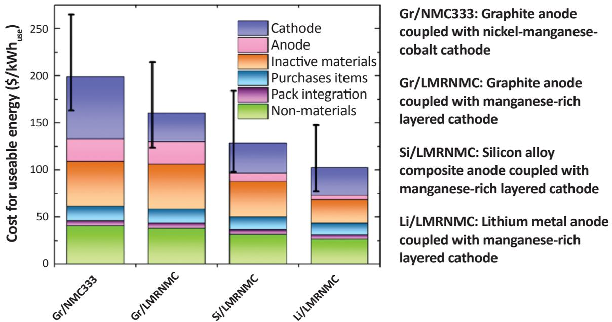
Estimated cost for a 100 kWh use PEV battery using advanced technology and produced at 100,000 packs per year. (Courtesy of Argonne National Laboratory, Joint Center for Energy Storage Research, supported by DOE Office of Science, Basic Energy Sciences.)
