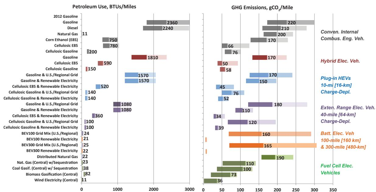
Diverse technology options exist to reduce transportation petroleum use and GHG emissions. The only options that achieve very high petroleum reductions and very low carbon emissions combine electric drive with low-carbon fuels. Contributions of vehicle cycle, fuel production, and vehicle operations are given in the Technology Assessments.<sup>11</sup>
