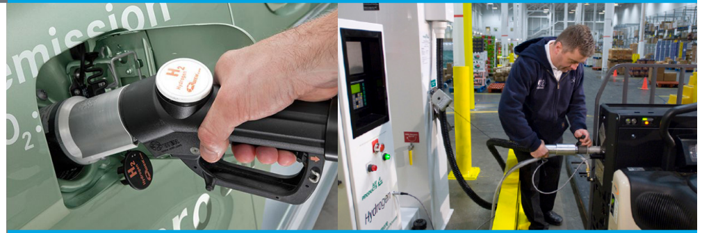
Like natural gas vehicles, fuel cell electric vehicles and material handling equipment are refueled with hydrogen using a closed-loop system to ensure safe operation.
