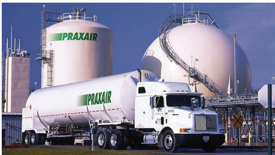
Gaseous hydrogen is liquefied by cooling it to below  $-253^{\circ}\text{C}$  ( $-423^{\circ}\text{F}$ ). Once hydrogen is liquefied it can be stored at the liquefaction plant in large insulated tanks.
