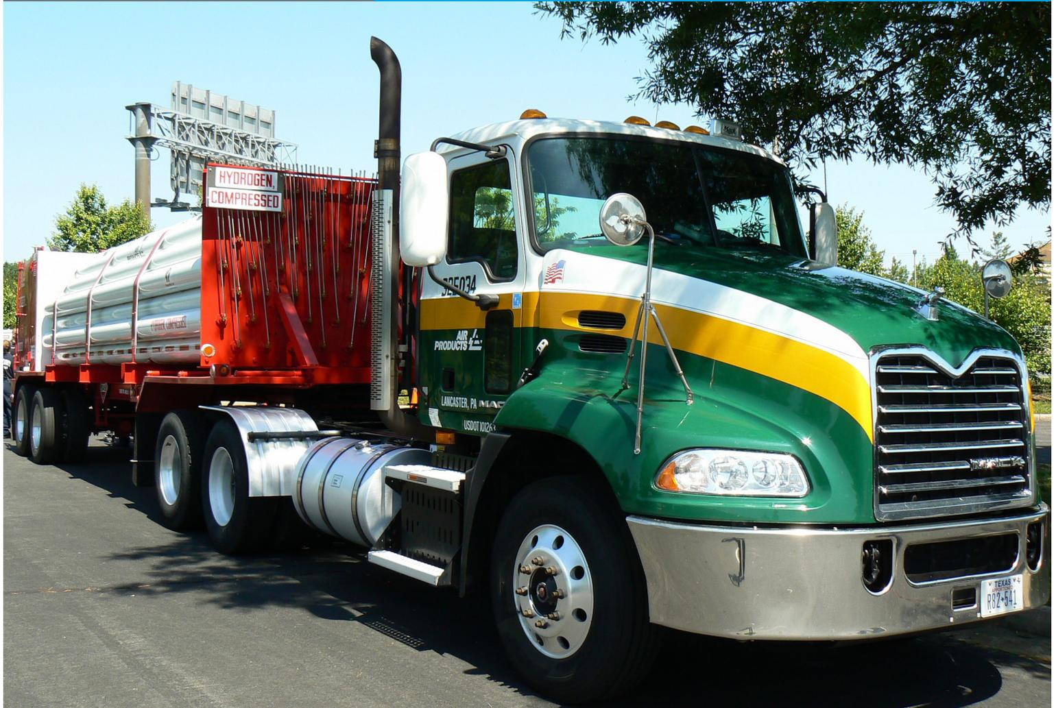
A viable hydrogen infrastructure requires that hydrogen be able to be delivered from where it's produced to the point of end-use, such as a dispenser at a refueling station or stationary power site.
