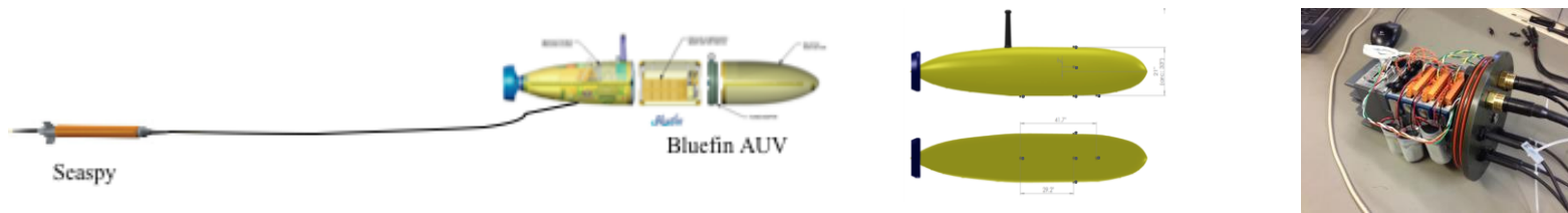
Fig. 2 EMF measurement system (a) schematics of towing of SeaSpy magnetometer from the Bluefin AUV, (b) location of E-field sensors on AUV hull, (c) E-field acquisition and processing unit
