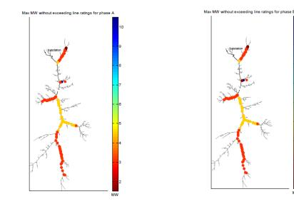
Figure 112. Maximum wind power at a bus that does not exceed line ratings for Phase A
