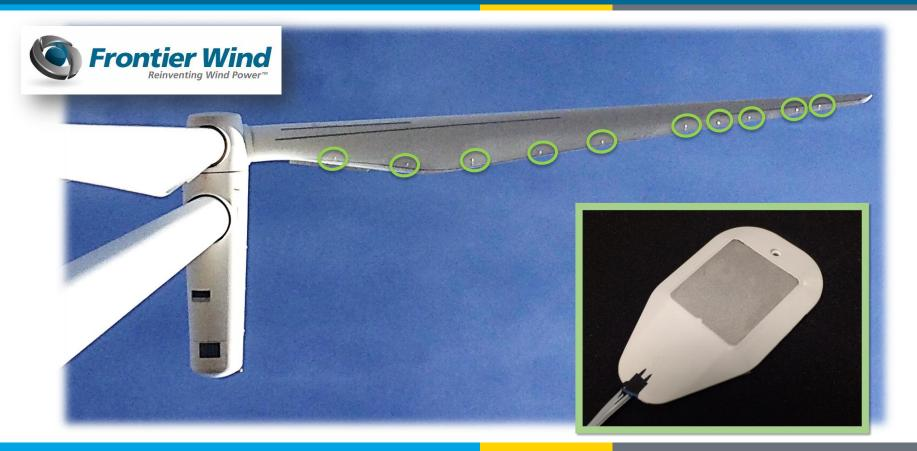
Rotor-Mounted Bat Impact Mitigation System
