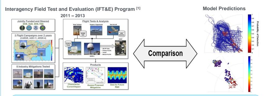
Assess radar model wind turbine impact predictions using real-world data collected during the Interagency Field Test & Evaluation (IFT&E) Program
