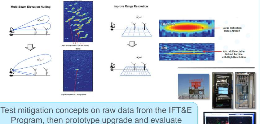
performance at radar sites with real-time testbed
