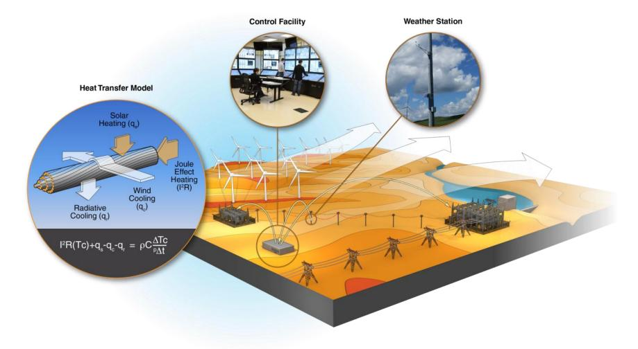
Use computational fluid dynamics and real-time weather data to deploy an industry standard line rating methodology to open up marked increases in power carrying capacity of existing overhead lines and seamlessly implement it into the control room.
