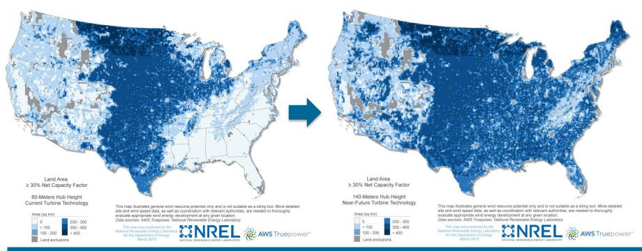
Example: R&D enabling cost-effective "tall wind" technologies (150 W/m<sup>2</sup> specific power rotors at 140m hub height) would increase land area with  $\geq$  30% net capacity factor by 67% and open substantial development opportunities in all 50 states. Zayas et al. (2015), *Enabling Wind Power Nationwide*
