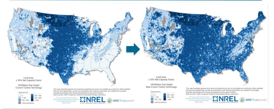
Example: R&D enabling cost-effective "tall wind" technologies (150 W/m<sup>2</sup> specific power rotors at 140m hub height) would increase land area with  $\geq$  30% net capacity factor by 67% and open substantial development opportunities in all 50 states. Zayas et al. (2015), *Enabling Wind Power Nationwide*
