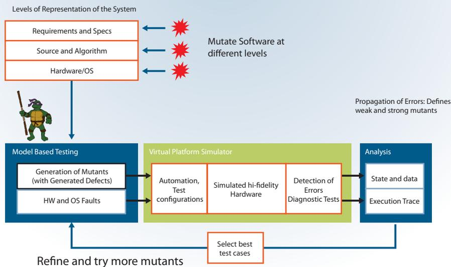
**Figure 1. Virtualized mutation testing: simplified view.**
