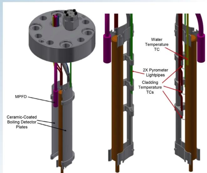
**Figure 3. Instrumentation design for each Multi-SERTTA capsule. (Left) Head unit assembly, (middle) right view of hangar rod showing IR pyrometer light pipes, (Right) left view showing thermocouples.**
