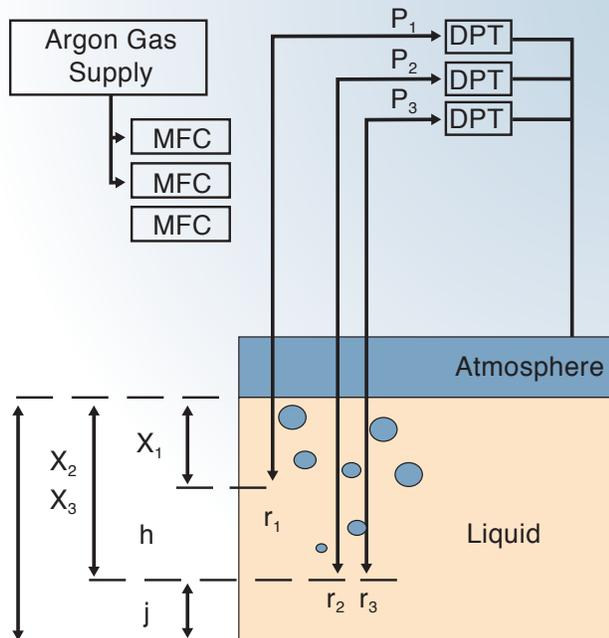
Figure 1. Schematic of the triple bubbler system
