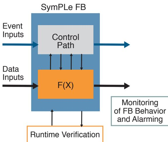
Figure 3. SymPLe Function Block Design.
