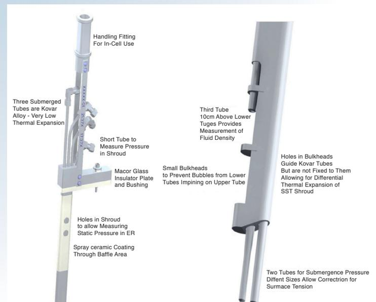
Figure 2. 3D rendering of the triple bubbler system probe.
