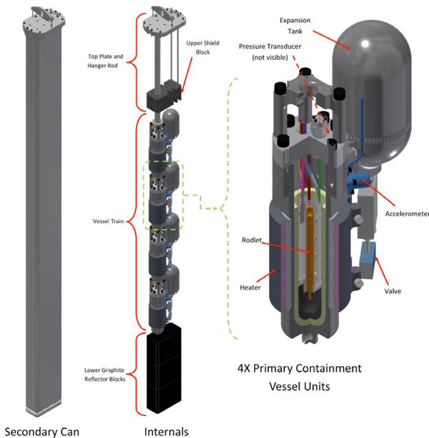
**Figure 2. Rendering of the Multi-SERTTA vehicle for testing fuel rodlets under transient overpower conditions corresponding to high temperature and high pressure conditions of Pressurized Water Reactors (PWR). Based on successful experiment devices of the past, the design is a “package”-type loop incorporating experiment containment and supporting instrumentation in a single box that displaces TREAT fuel elements in the center of the core.**
