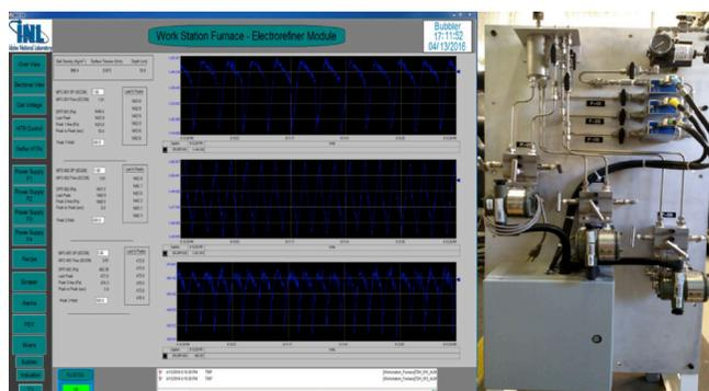
**Figure 4. (left) Data acquisition control and (right) the bubbler instrument panel.**
