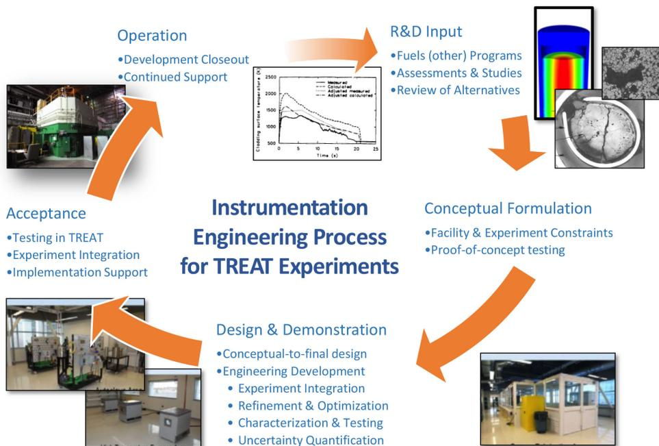
**Figure 5. Instrumentation development process for experiment deployment.**
