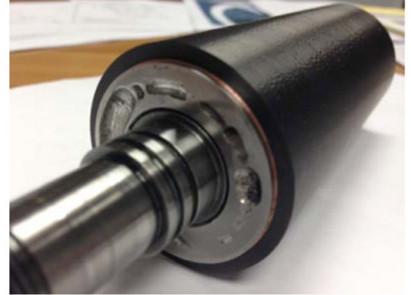
Left: Visual of benefits of integrated variable speed drive and high-speed megawatt motors for gas compression. Right: A Calnetix rotor with the type of composite fiber carbon fiber sleeve and copper shielding to be used in the high-speed motor. Images courtesy of Eaton
