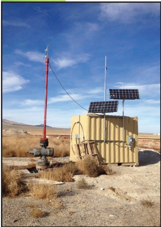
The RRG-9 ST-1 wellhead fitted with a lubricator. A distributed temperature sensor was run through the lubricator to measure well bore temperatures. Photo source: Energy & Geoscience Institute at the University of Utah.
