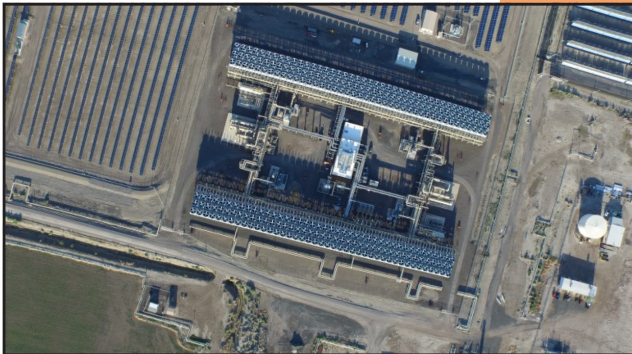
Engineers added a 2MW solar thermal power plant to support the existing geothermal plant. The thermal energy increases the temperature of the geothermal fluid entering the plant, increasing overall output.
