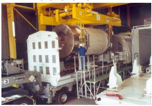
Fig. 2-8. TN 52L dual-purpose SNF cask being loaded onto a heavy-haul road vehicle (Roland 2001).
