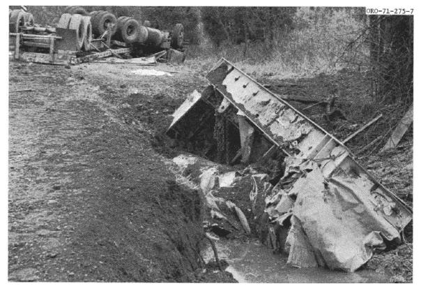
Fig. 4-2. Cask separated from tractor-trailer (Chandler 1972).
