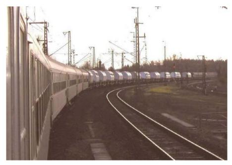
Fig. 2-14. Train consist containing 12 cask railcars and associated security personnel cars (Verdier 2004).
