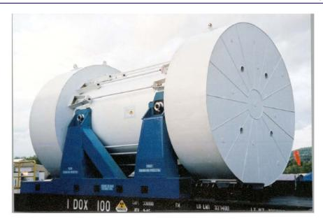
Fig. 2-16. Loaded West Valley cask with impact limiters and tie rods installed (Tyacke 2004).
