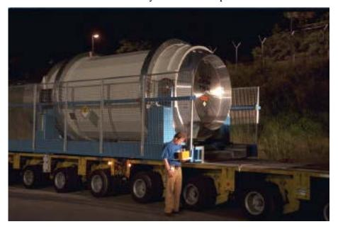
Fig. 2-10. The TN 97L dual-purpose cask loaded on a heavy-haul road transport vehicle (Sicard 2001).
