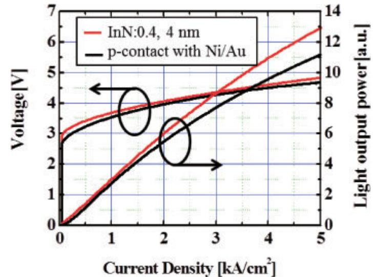
The same characteristics:  $r_s = 2.3 \times 10^{-4} \Omega\text{cm}^2$
