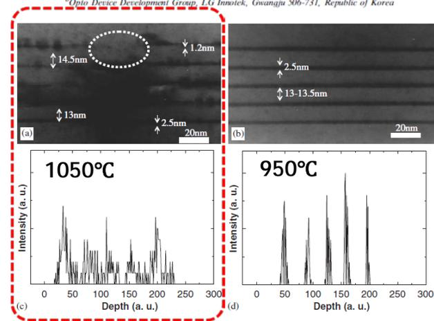
n-GaN/tunnel junction/p-GaN grown at low temperature could be a solution.
