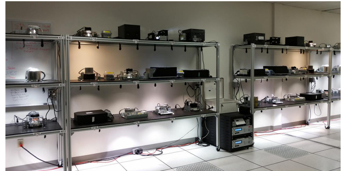
Figure 1. A portion of the downlight test racks in operation. A total of six racks house 70 luminaires.
