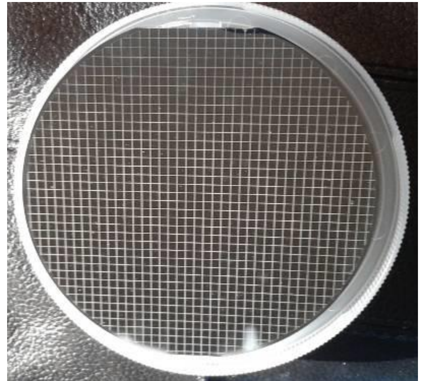
150mm diameter 3C-SiC on (001)Si
