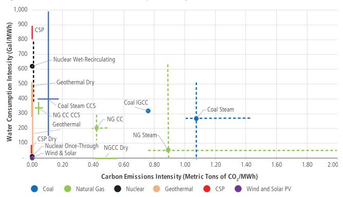
Figure 3-26. Carbon Emissions and Water Consumption Intensity Tradeoffs<sup>339, 340, 341, 342, 343, 344</sup>
