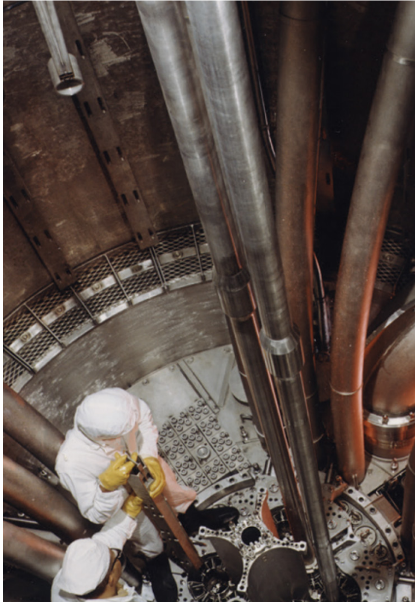
Advanced Test Reactor (No. 3) is used to study the effects of radiation on materials and is also capable of producing rare and valuable medical and industrial isotopes. It is the most versatile test reactor in the world.
