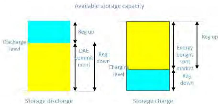
**Figure 3-2 Regulation up and down during charging and discharging**
