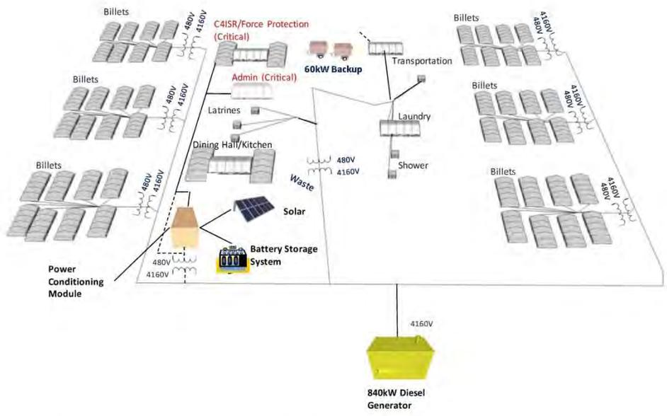
**Figure 2: 550-person Battalion: 1 Generator with energy storage and alternative energy generation**
