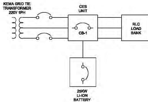
Fig 2. Test Set up with load bank.
