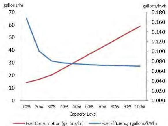
Figure 4: Fuel consumption and efficiency of 840 kW generator
