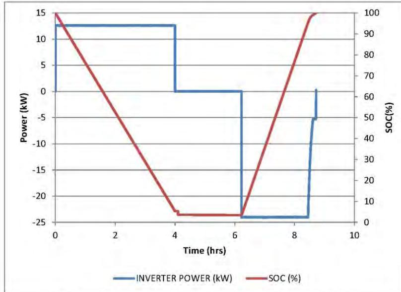
Figure 4f. Second peak shaving profile test at 12.6 kW discharge
