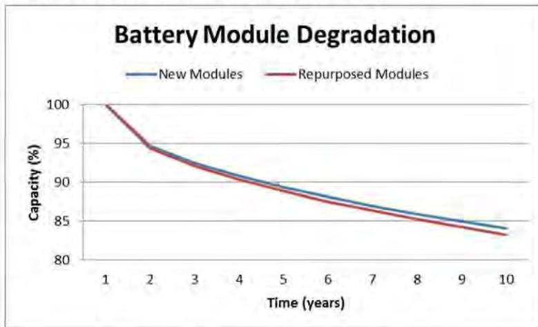
Figure 3-3 Battery Module Degradation for Peak-Shaving
