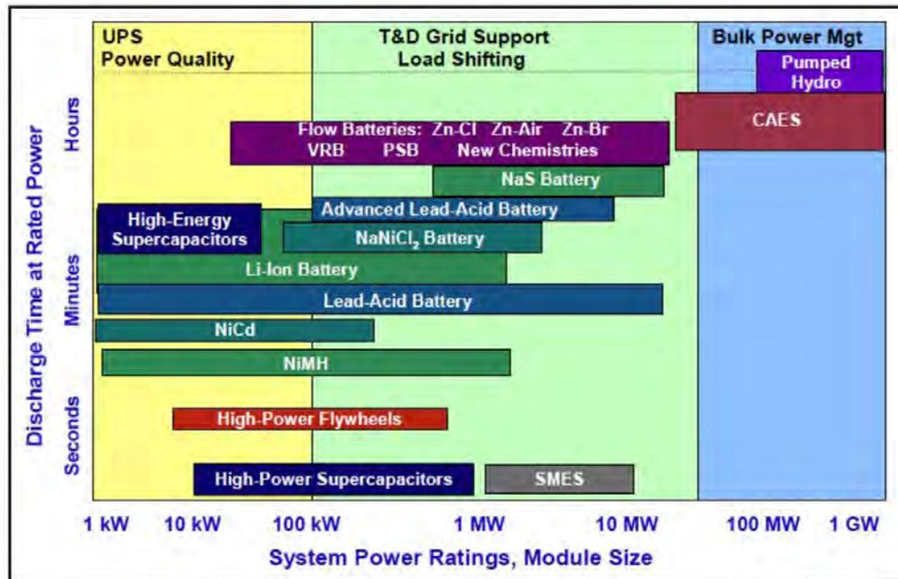
Figure 3: Positioning of Energy Storage Technologies
