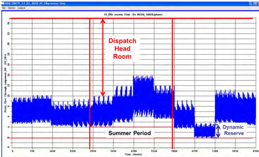
**Figure 12: Transformer Loading Identifying Dispatch Headroom**
