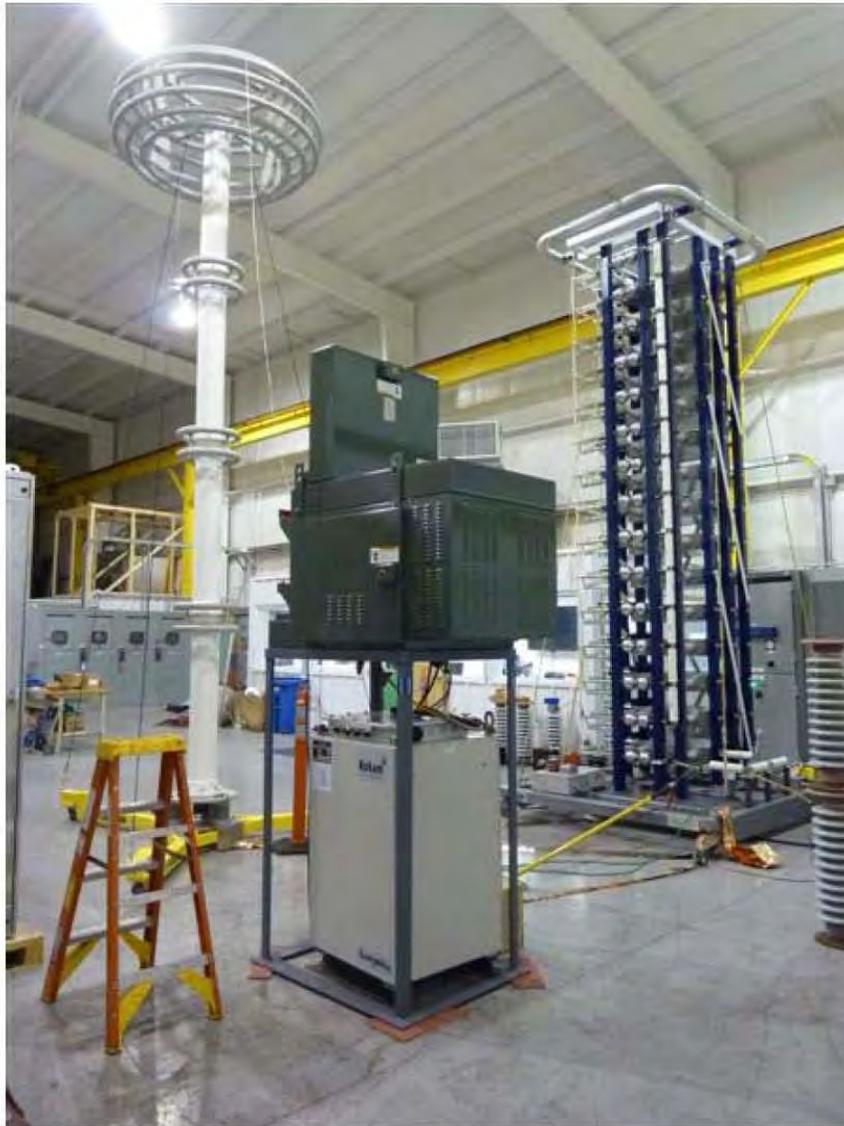
Set up for BIL test. CES unit and battery on test stand. KEMA Impulse generator is the blue rack to the right and white voltage divider on the left.
