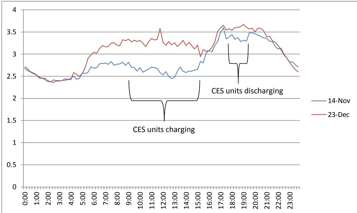
Summary - The Renewable Energy Time Shift can be configured to shift a portion of the PV production to the time when the circuit peak normally occurs. The result is similar to a static peak shaving application.
