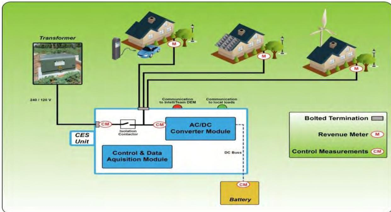
**Figure 3: CES Application Diagram**
