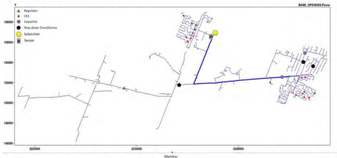
**Figure 3-1 OpenDSS Trinity Circuit Diagram**
