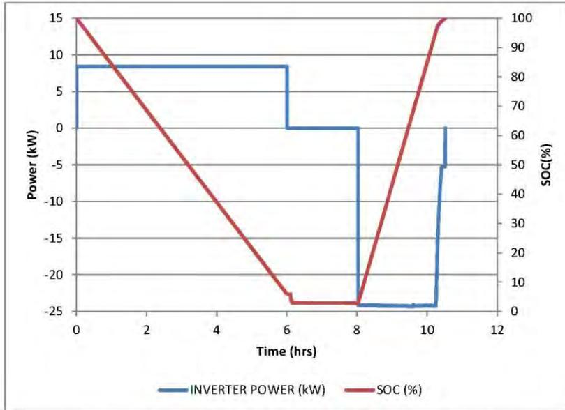
Figure 4d. Second peak shaving profile test at 8.4 kW discharge
