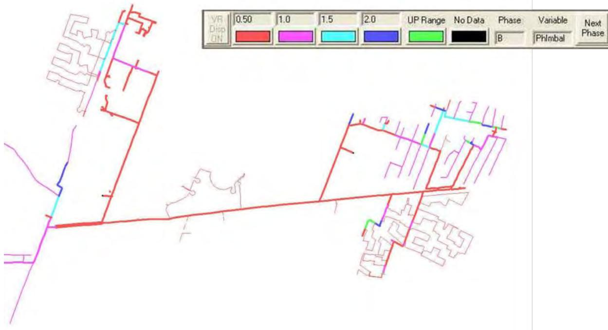
**Figure 15: Circuit Model Identifying Phase Imbalance**
