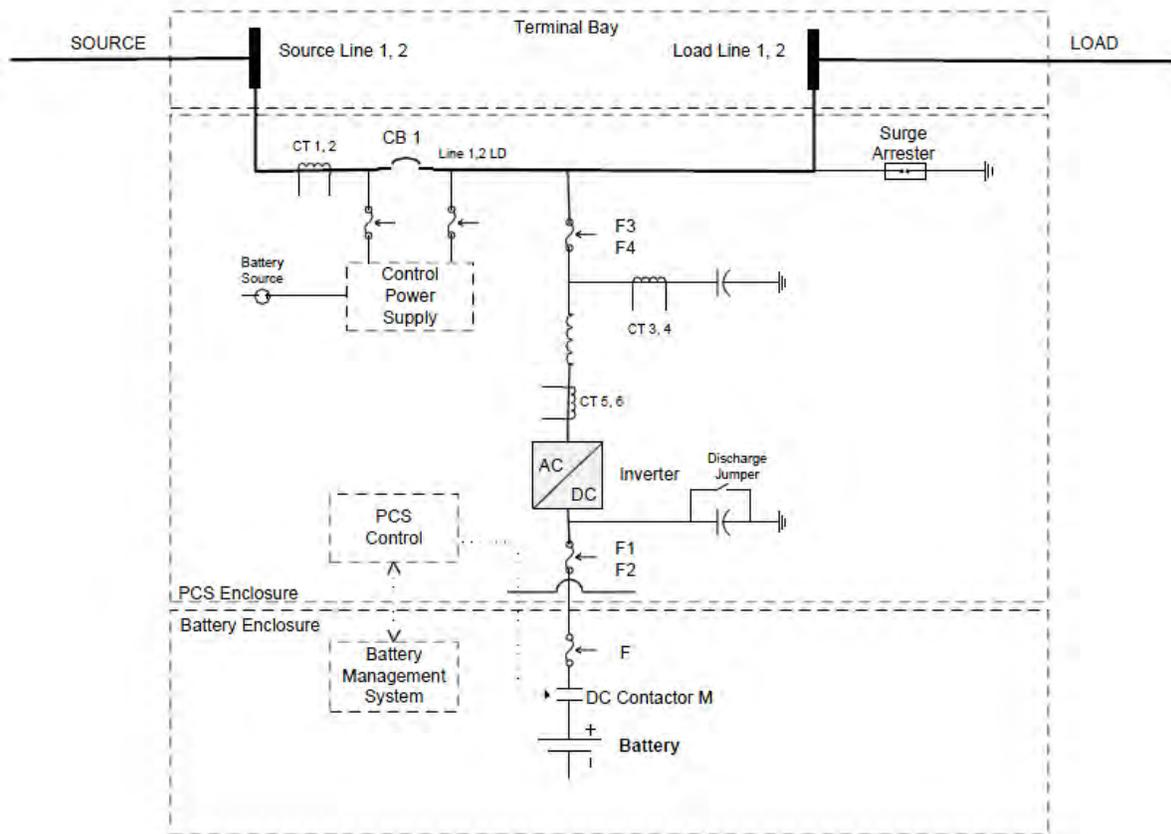
**Figure 4: CES Electrical One Line Diagram**
