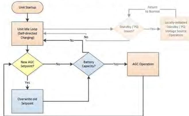
**Figure 3-3 Frequency Regulation control logic**
