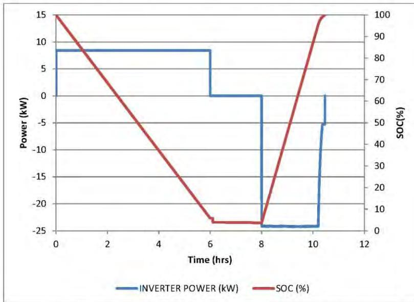
Figure 4c. First peak shaving profile test at 8.4 kW discharge
