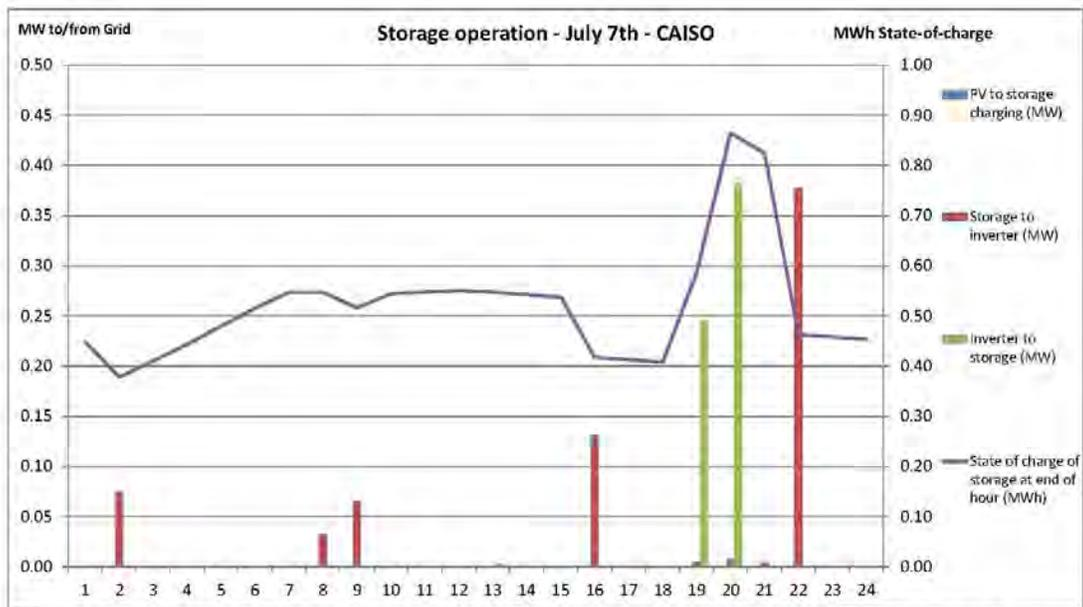
**Figure 4-9 Storage Dispatch and State-of-Charge for CAISO Market Case with New Battery Modules - July 7<sup>th</sup>**
