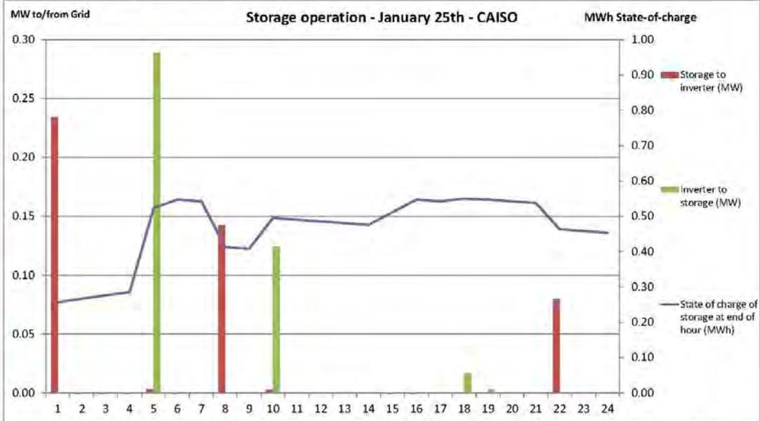
**Figure 4-11 Net Storage Dispatch and State-of-Charge for CAISO Market Case with New Battery Modules - January 25<sup>th</sup>**
