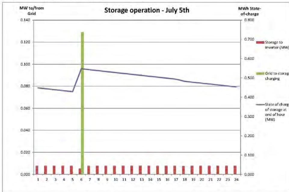
**Figure 4-2 Net Storage Dispatch and State-of-Charge for MISO Market Case with New Battery Modules – July 5<sup>th</sup>**
