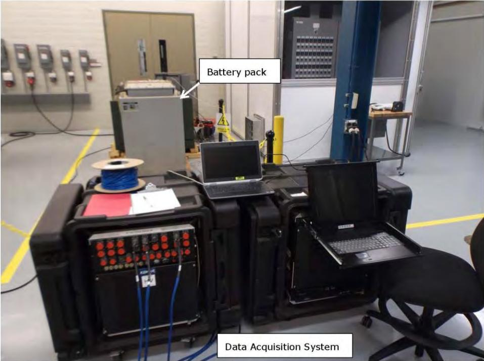
Figure 10. Data acquisition system
