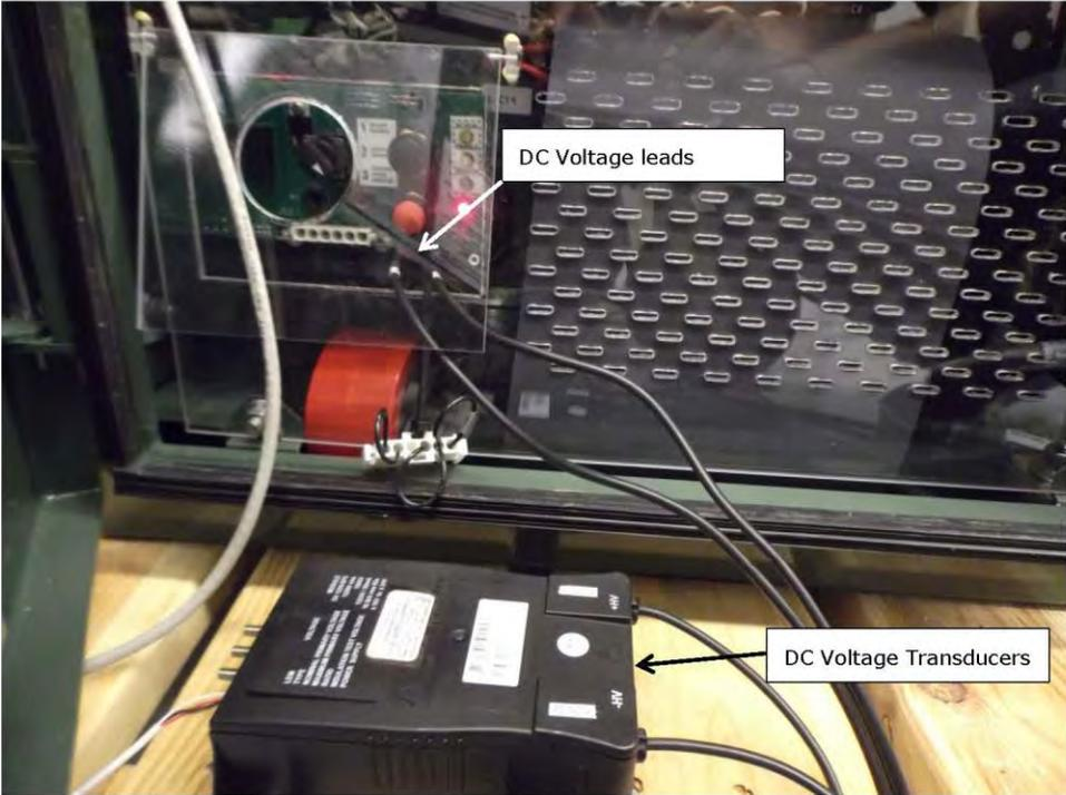
Figure 8. DC voltage measurement setup
