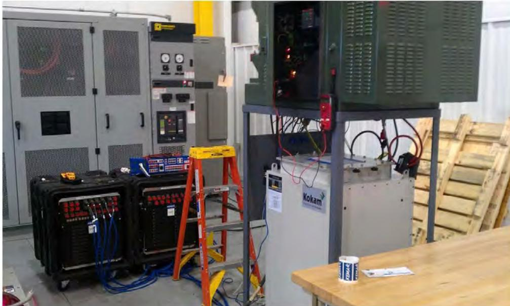
CES on stand with battery under. KEMA Power transformer in back. DAS, Blue cables to V and C transducers.
