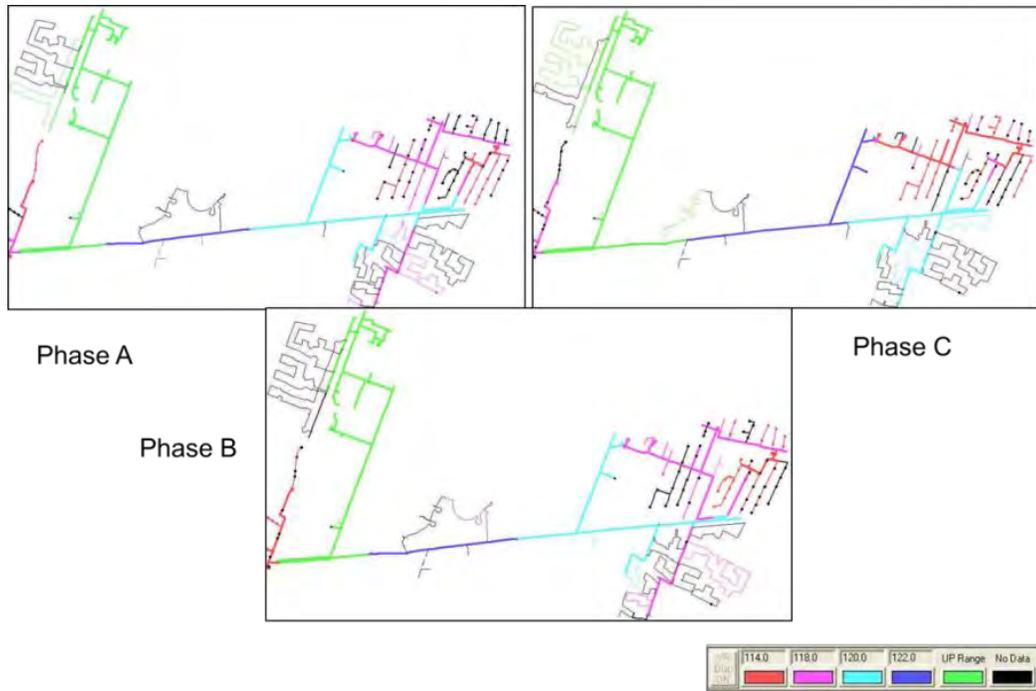
**Figure 13: Circuit Model Identifying Phase Voltage for CES Placement**
