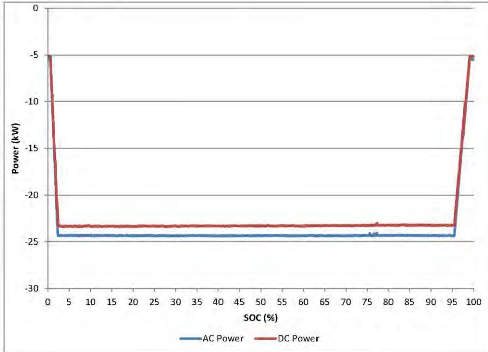
Figure 1. Charge power vs. battery state of charge
