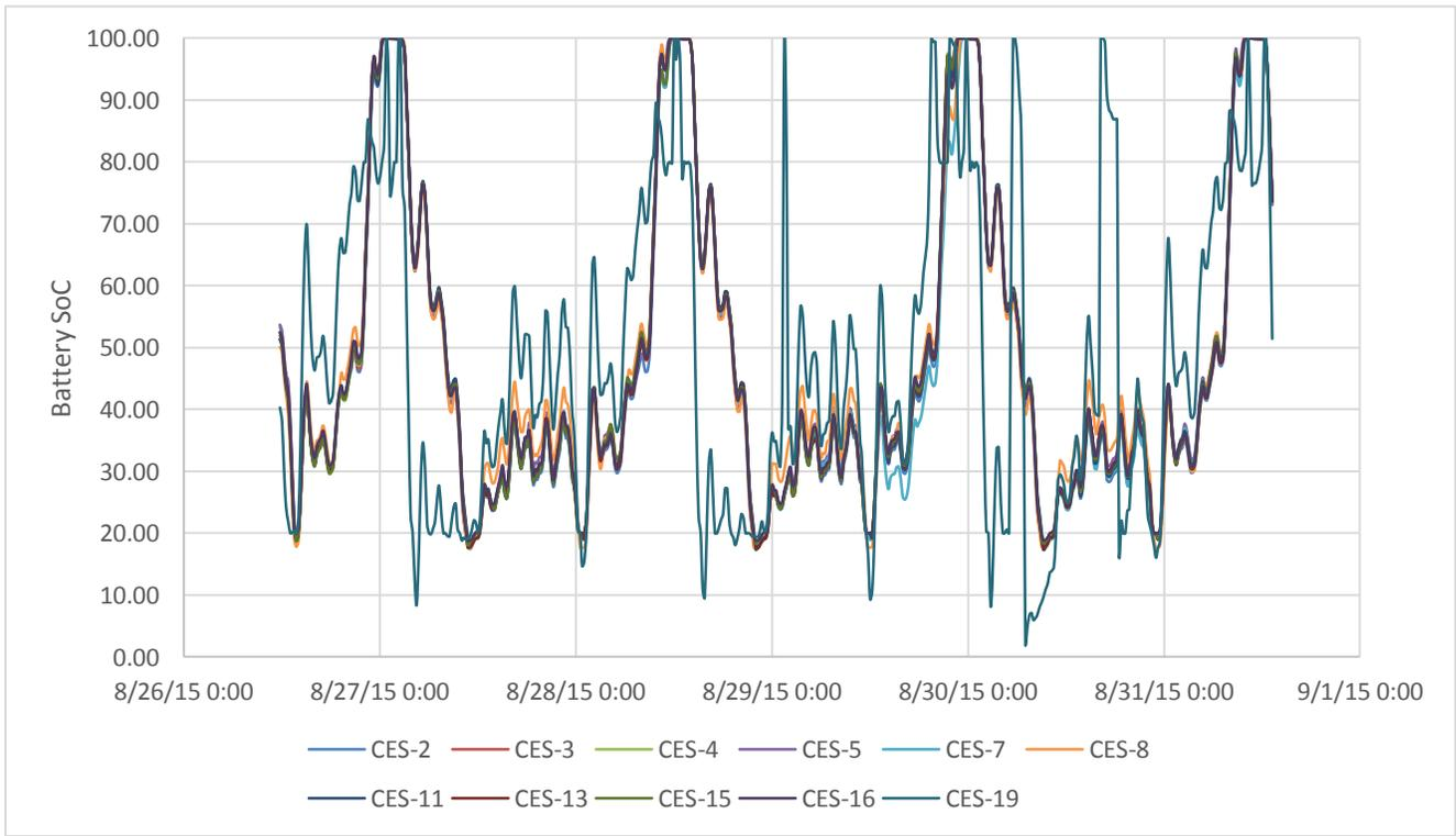
CES-19's deviance appears to be the result of the way the SoC is computed in the repurposed battery. As with all of the CES units involved in this test, CES-19 was configured with a 20% reserve margin. Each time the repurposed battery reported a SoC value below this threshold, its inverter immediately started a maintenance charge. This behavior explains the downward spiking and the prompt recovery observed in the results.
