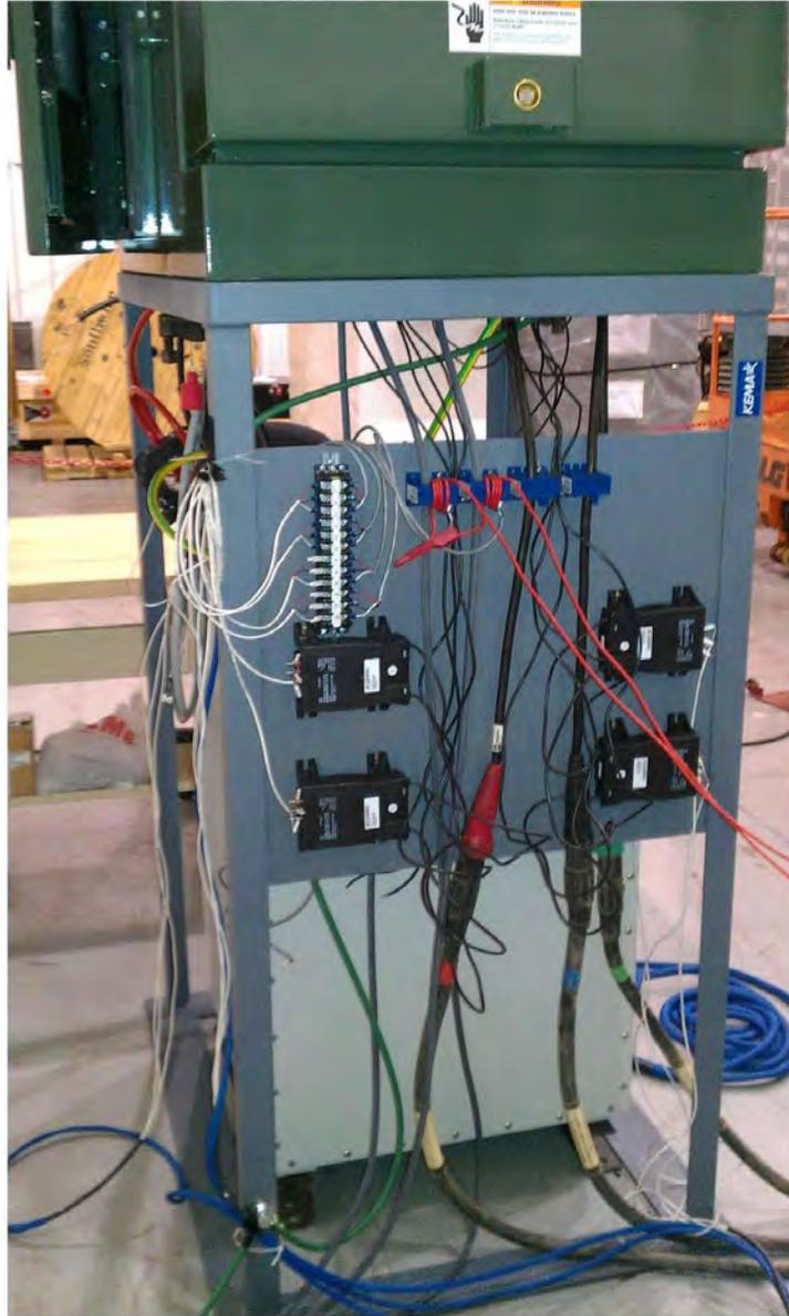
KEMA CES test stand. Source current(blue) and source voltage(black) transducers to the left and load current and voltage transducers to the right. Large power cables go to load bank.
