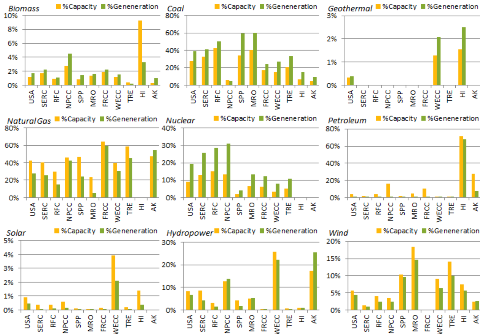
Figure 4-21. Capacity and generation shares for generation technologies and region
