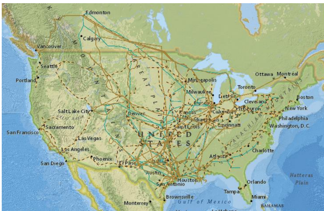
Figure 13-7. Pipelines in the U.S. and Canada that transport petroleum products
