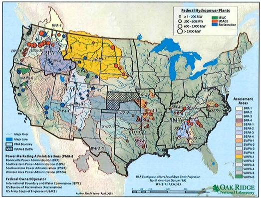
Figure 1. Federal hydropower facilities and power marketing regions in the United States. Note that part of Kansas is supplied by both WAPA and SWPA.
