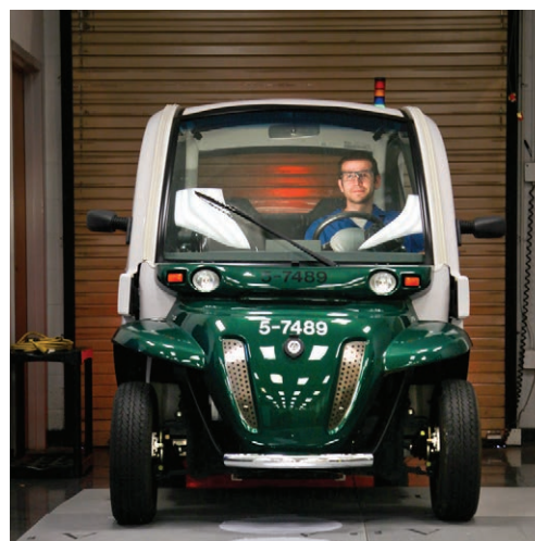
Researcher demonstrates an electric vehicle being wirelessly charged using ORNL technology at the National Transportation Research Center.
