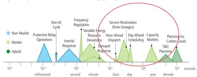
Figure 4-2. System Reliability Depends on Managing Multiple Event Speeds<sup>12</sup>
