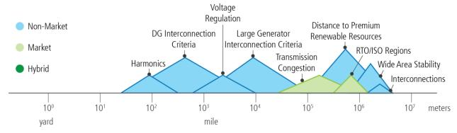
A variety of grid services are managed across different distance scales, and markets can be used to integrate some necessary services.
