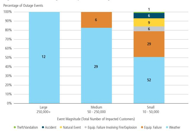
Figure 4-9. US Electric Outage Events by Cause and Magnitude, 2015<sup>97</sup>
