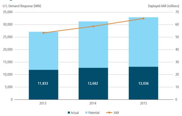
Figure 4-5. Advanced Metering Infrastructure Growth Has Contributed to Expanded Role of DR Programs<sup>69</sup>
