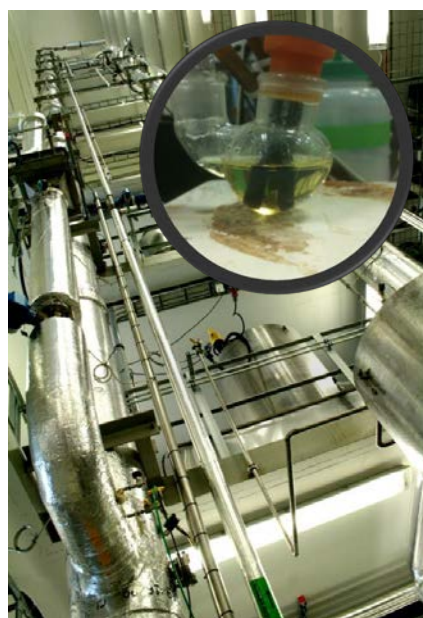
Figure 3: A Non-aqueous solvent (NAS) planned for testing at Tiller facility. The NAS will reduce water content and energy demand for regeneration as well as reduce the reactor size, resulting in better economics
