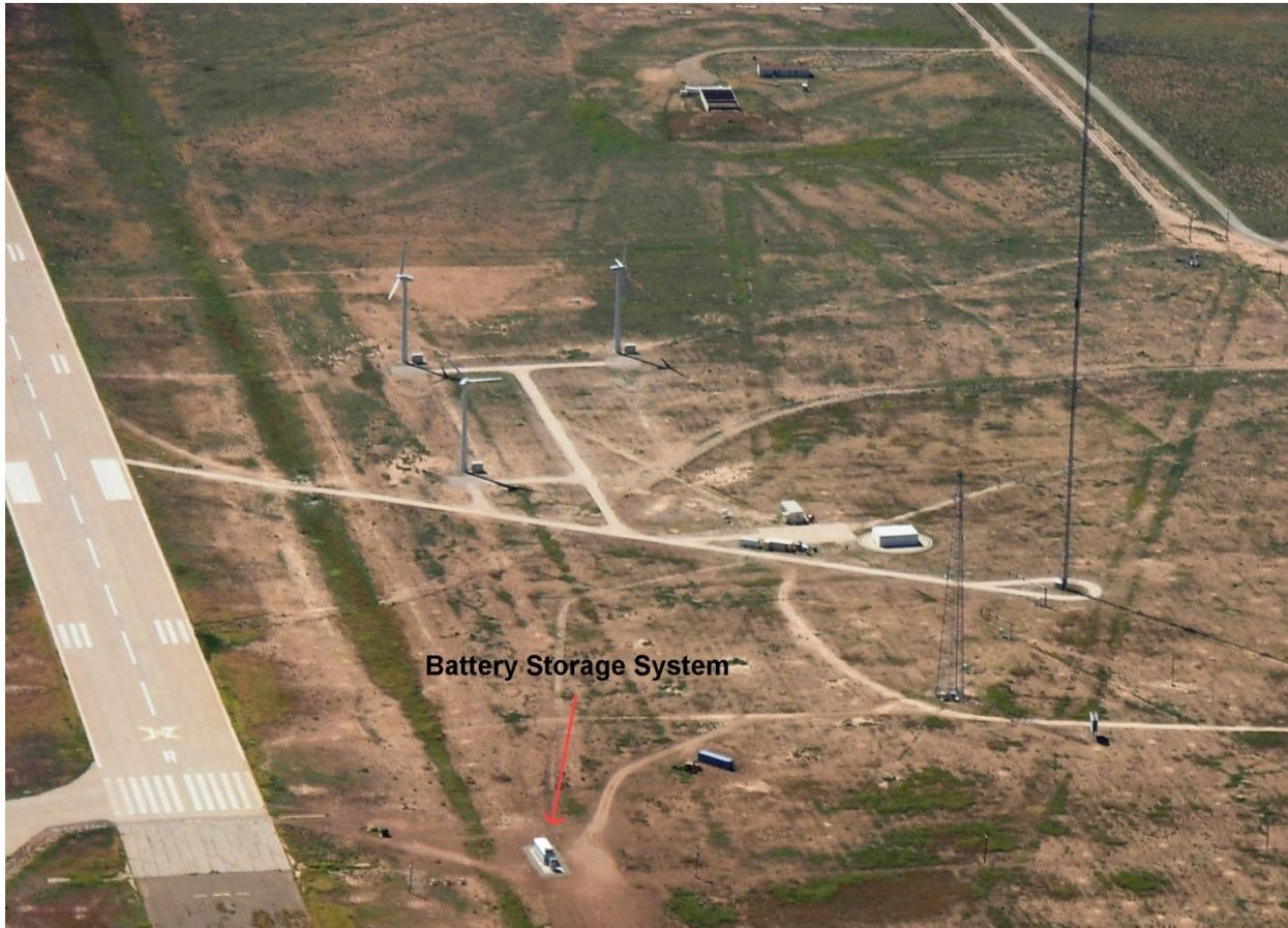
Figure 6. Aerial View of the BESS and the SWiFT Facility Turbines
