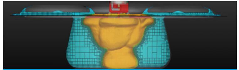
Fig 5. Simulation results for conventional, lean-burn spark ignition operation provide a baseline comparison for estimating potential efficiency and emissions benefits of reactivity controlled compression ignition. *Photo courtesy of Oak Ridge National Laboratory (ORNL).*
