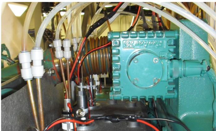
Fig 4. Laser igniters installed on a 6-cylinder engine. *Photo courtesy of Argonne National Laboratory.*
