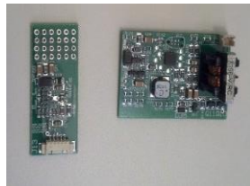
Gen 1 panel transceiver and driver
