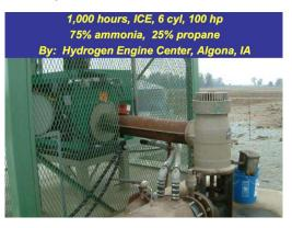
$NH_3$ -fueled ICE operating an irrigation pump in Central Valley, CA; ~ 50% total efficiency
