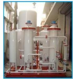
Ammonia cracking unit 200 nm<sup>3</sup>/h, 900 C, Ni catalyst
