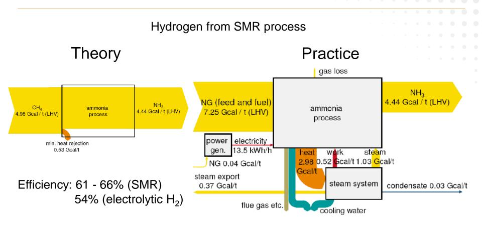
Energy consumption: 10000 - 12000 mWh/ton  $NH_3$  (current SMR) 6500 - 7500 mWh/ton  $NH_3$  (projected SSAS)
