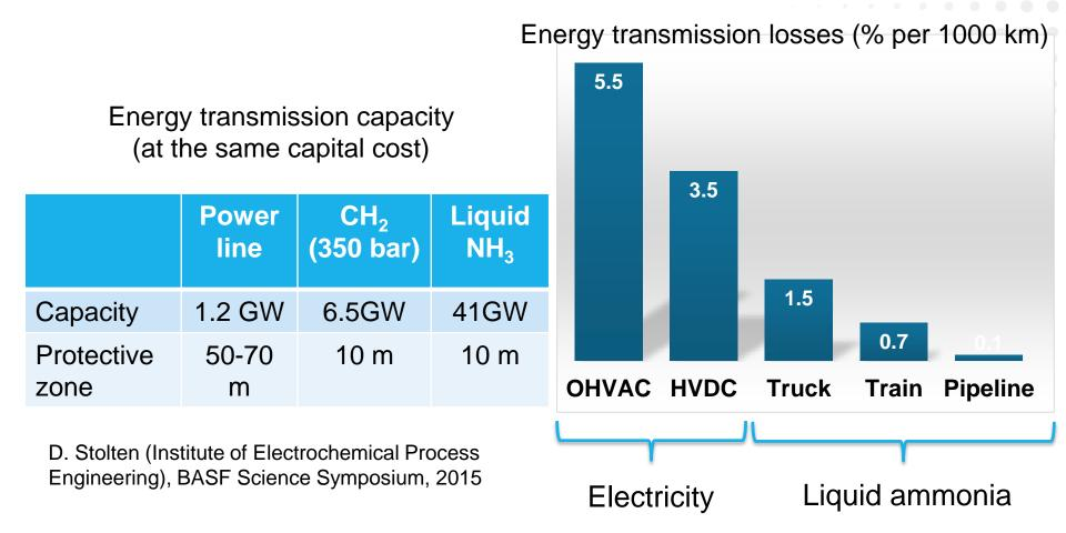
Liquid pipelines have highest capacity and efficiency
