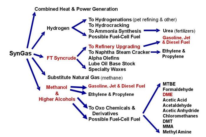
Molecules of H<sub>2</sub> and CO contained in synthesis gas are building blocks that can be used to synthesize a wide variety of complex hydrocarbons & organic compounds
