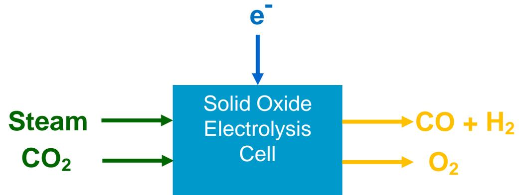
Industry-based co-electrolysis provide “negative” GHG emissions when producing fungible methanol.
