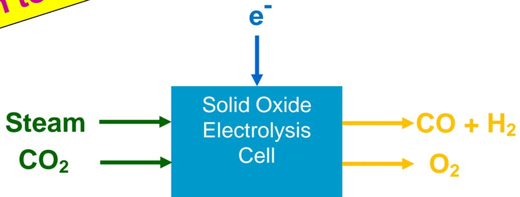
Industry-based co-electrolysis provide “negative” GHG emissions when producing fungible methanol.
