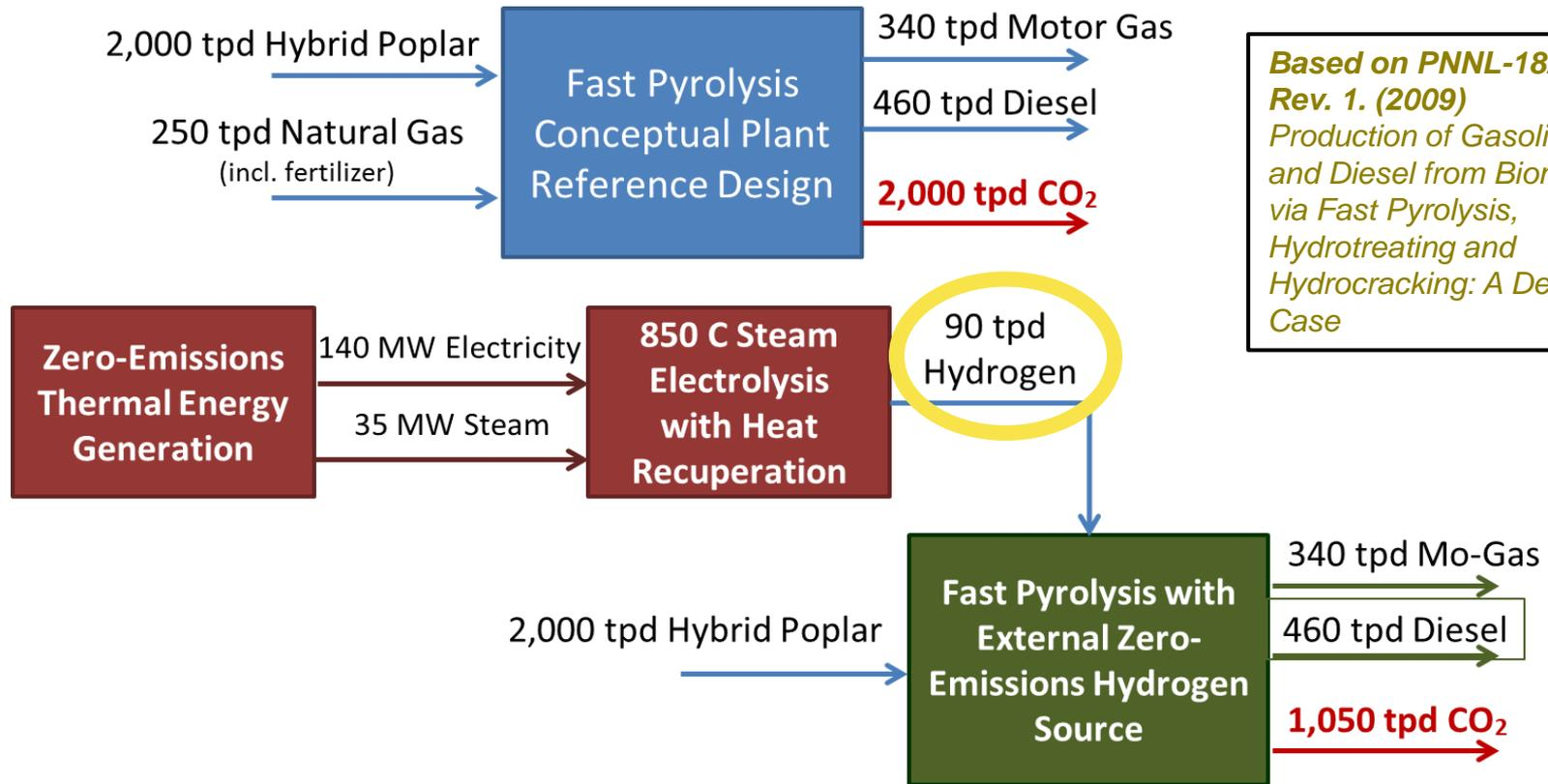
*Based on PNNL-18284 Rev. 1. (2009) Production of Gasoline and Diesel from Biomass via Fast Pyrolysis, Hydrotreating and Hydrocracking: A Design Case*
