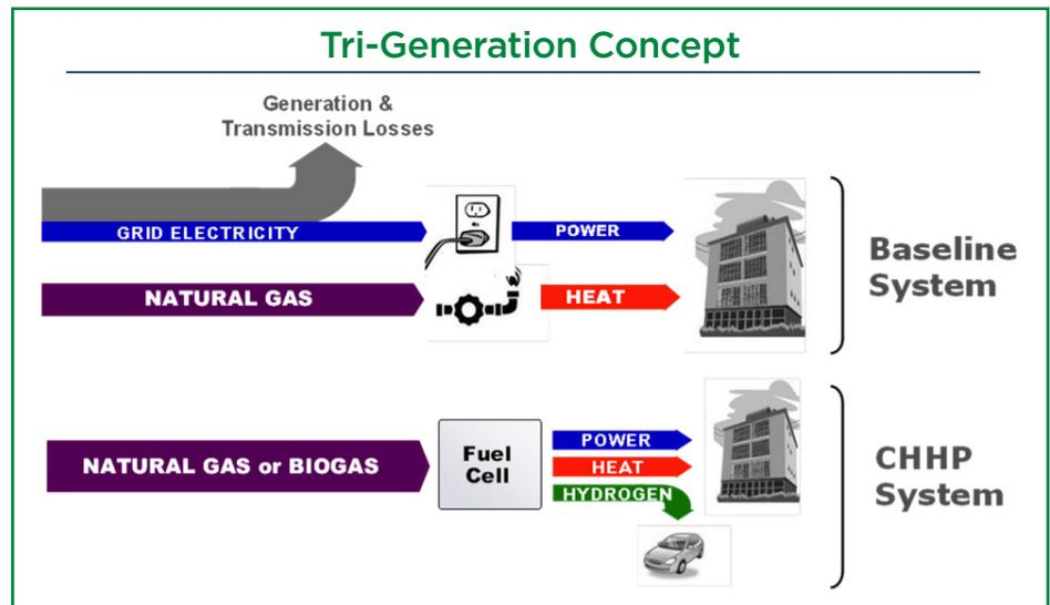
Tri-generation, or combined heat, hydrogen, and power (CHHP), systems can locally produce useful power, heat, and fuel with low emissions and high efficiency that avoids the energy and emissions penalties of transmission/transportation of traditional methods.
