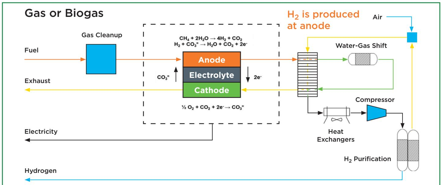
Anaerobic digester gas fuel is cleaned and then sent to a molten carbonate fuel cell that converts the hydrocarbons to a hydrogen rich mixture and produces electricity. Careful design modifications allow extra production of hydrogen that is separated, compressed, and dispensed to fuel cell vehicles.
