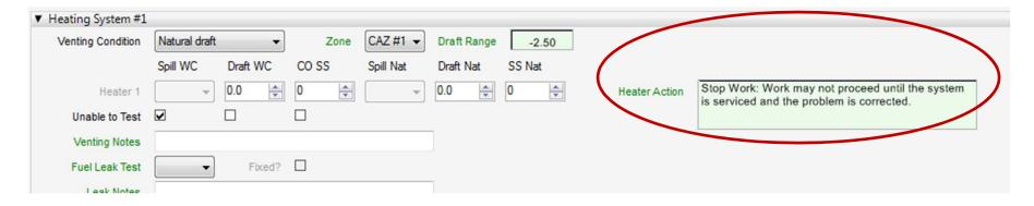
Ambient condition testing and required plan of action
