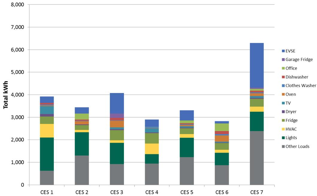
**Figure 11: Control Block Energy Use Breakdown (July 1, 2013 to February 28, 2014)**
