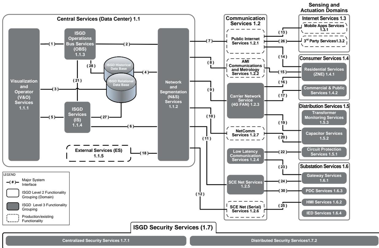
Decomposing the ISGD services domains into more discrete services, defining their requirements, and preparing detailed designs for each component provided the basis for selecting systems, equipment, and applications. Designs were prepared for each component, including processing, storage, and communications.
