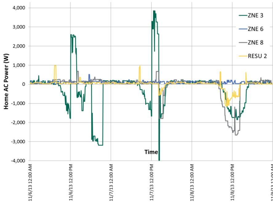
ZNE 6 stopped operating and communicating on November 6, 2013. As such, this RESU did not receive the DR event, and did not operate at all during the test. This was confirmed with the very low power recorded (between 0 and 500 W) which is attributable to this RESU's secure loads.
