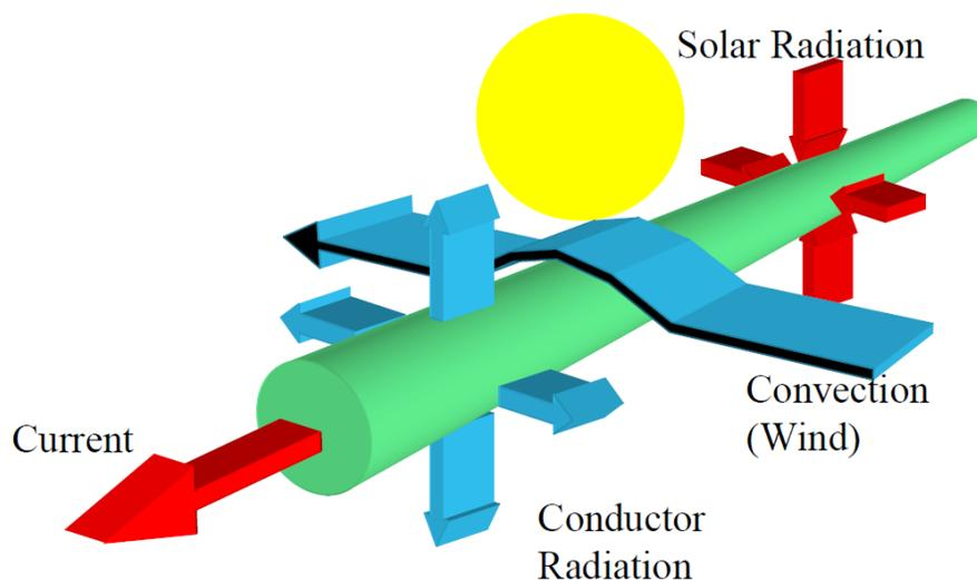
**Figure 4 - Conductor Line Rating Thermal Characterization**
