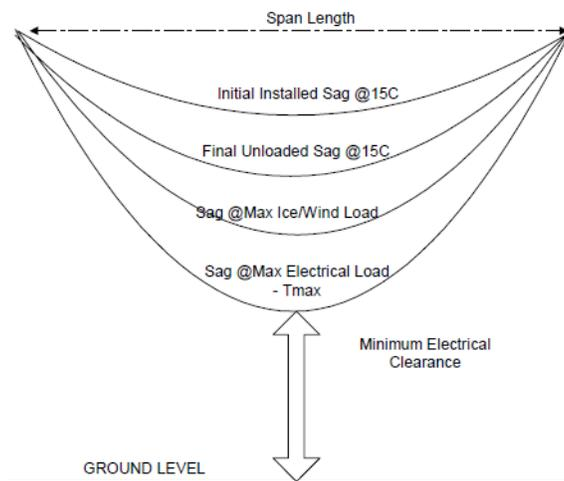
**Figure 7 - Typical set of sag curves for a span**
