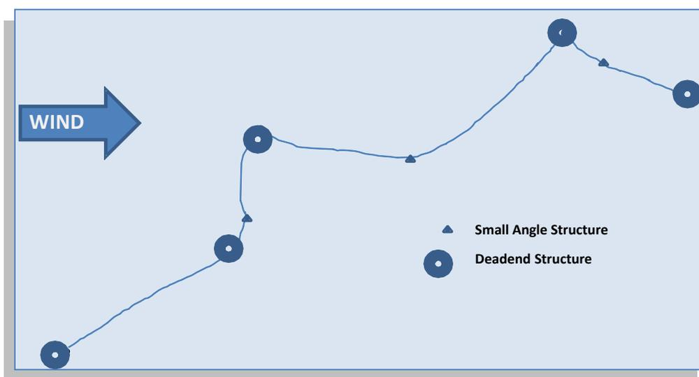
Figure 12 – Simple Transmission Line Layout
