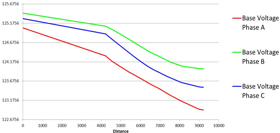
Figure 34 - Voltage Profile with the Traditional Method
