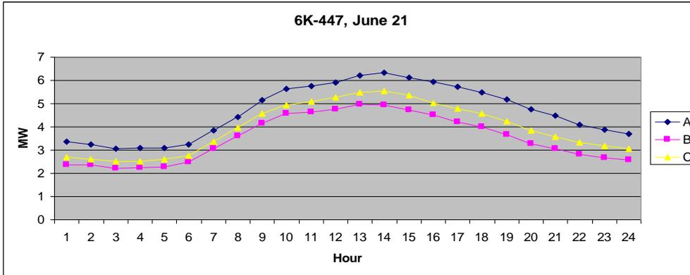
Figure 26 - Load Shape of 6K-447 on June 21, 2012
