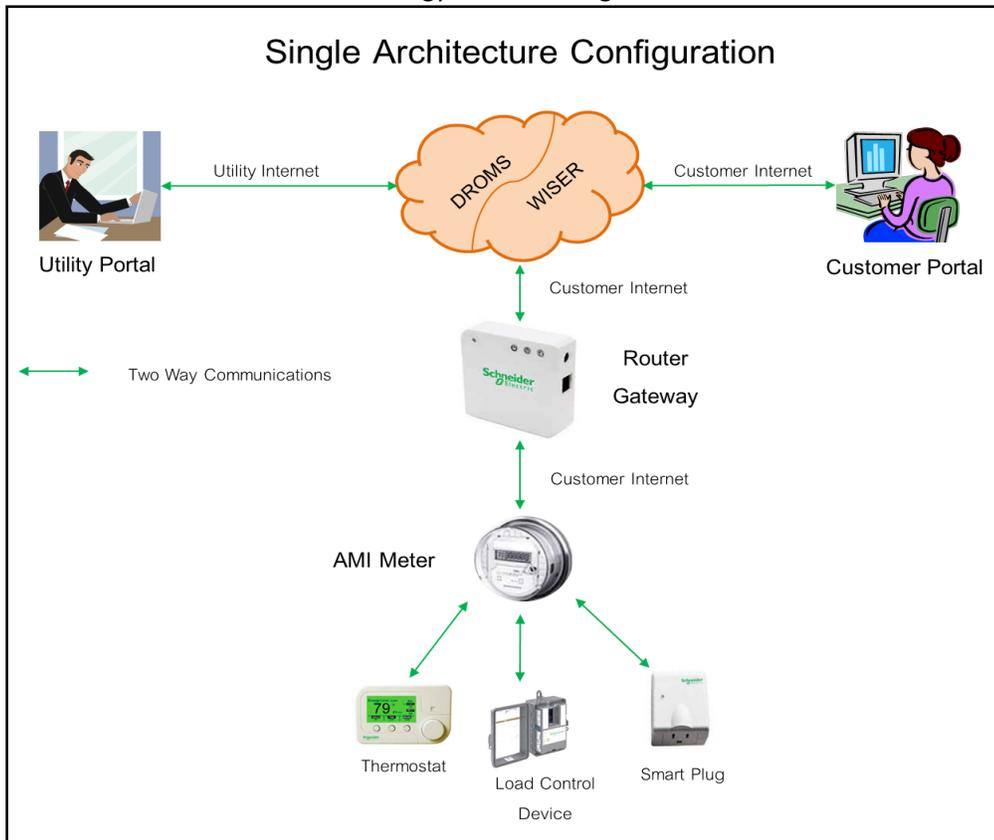
Figure 15 – PSEG Long Island DLC System Single Architecture
