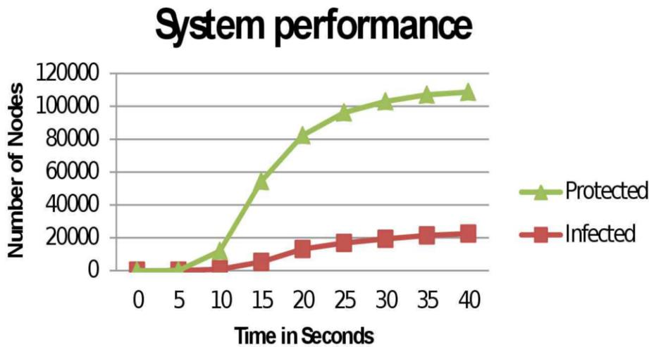
Figure 39 - Number of Nodes Protected and Infected in Simulations of Our Network Defense
