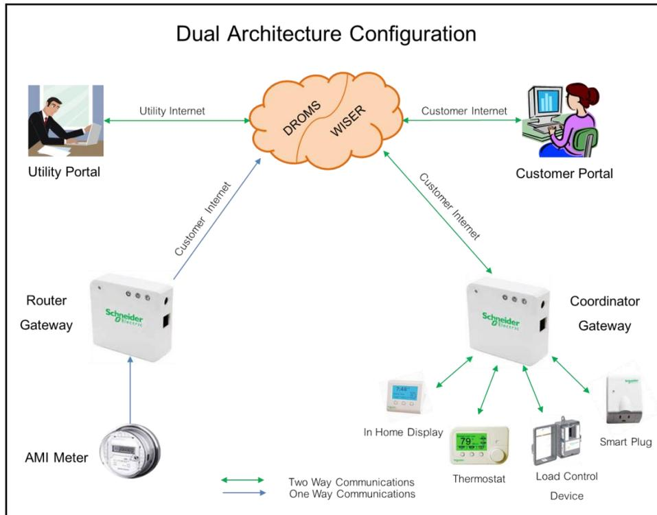
Figure 17 – PSEG Long Island DLC Dual System Architecture
