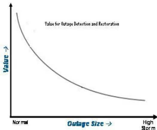
Figure 22 - Relationship between Outage Detection and Outage Size
