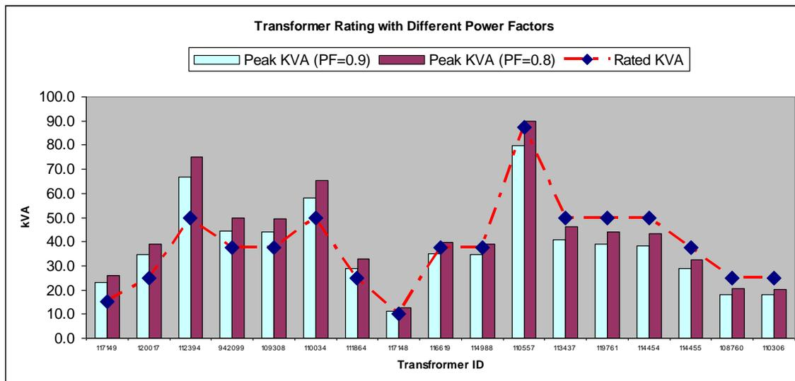
Figure 28 - Transformer Rating with Different Power Factors
