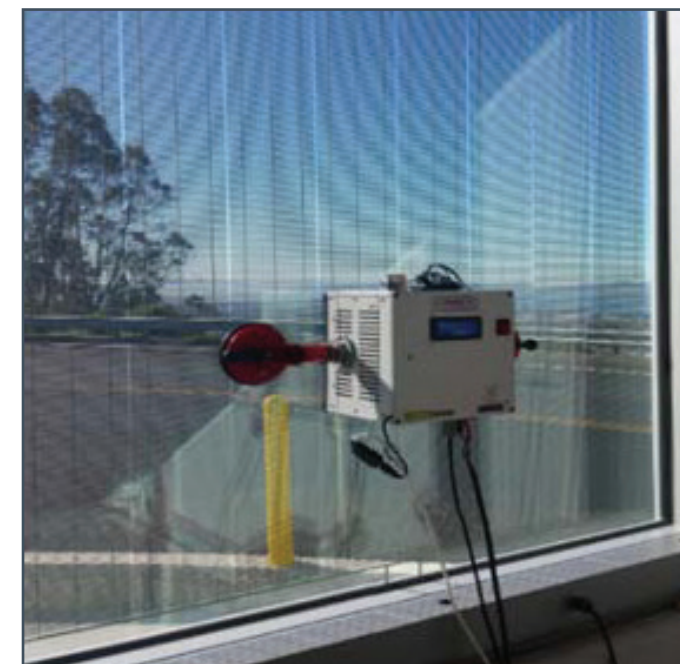
Portable Window Energy Meter (prototype)—jointly developed by Brazil Federal University of Santa Catarina and U.S. Department of Energy Lawrence Berkeley National Laboratory under the U.S.-Brazil Strategic Energy Dialogue.
