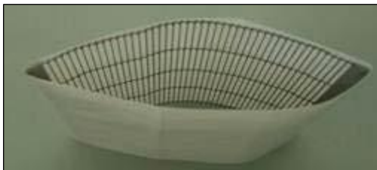
Figure 136. Plate Frame Membrane Humidifier single cell pouch (Source: Johnson, William B. "Materials and Modules for Low-Cost, High Performance Fuel Cell Humidifiers," W.L. Gore & Associates, Inc., presentation at the 2012 DOE Hydrogen and Fuel Cell Program Annual Merit Review, Washington, DC, 17 May 2012.)
