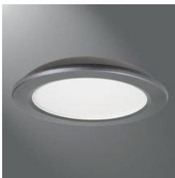
18" diameter, 4.5klm output 1cm thick; enabled by: CSP LEDs + Lightguides
