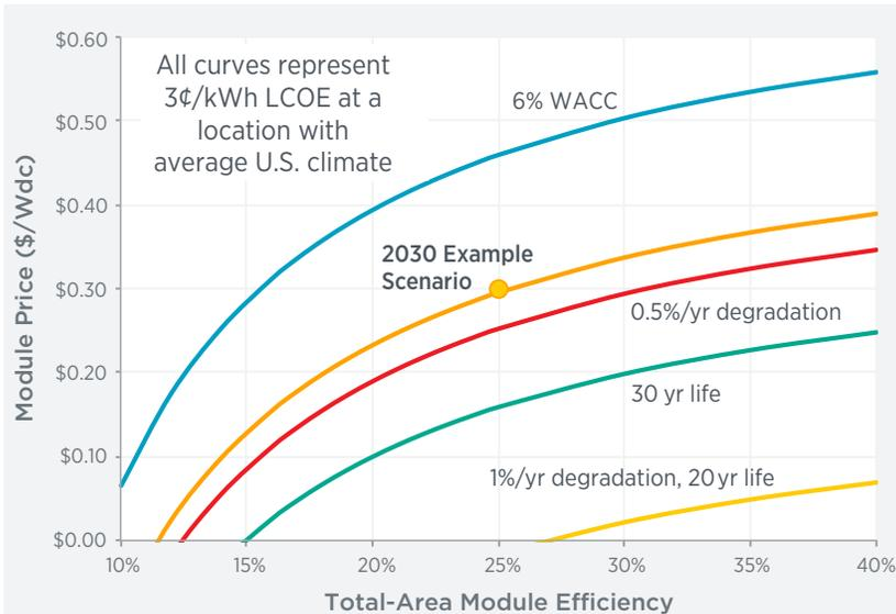
**Figure 4. Curves illustrating numerous module technology pathways to reach the SunShot 2030 utility-scale goal.** Every point on each curve corresponds to a 3¢/kWh LCOE. Unless otherwise noted, all scenarios assume one-axis tracking systems with 1,860 kWh(AC)/kW(DC), five-year MACRS, 7% weighted average cost of capital WACC), 2.5% inflation, \$0.85/W system cost, \$4/kW-year O&M, 0.2%/year degradation and a 50-year system lifetime.
