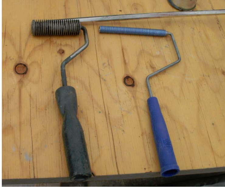
Figure 18B – Serrated Metal Rollers for Installation Process
