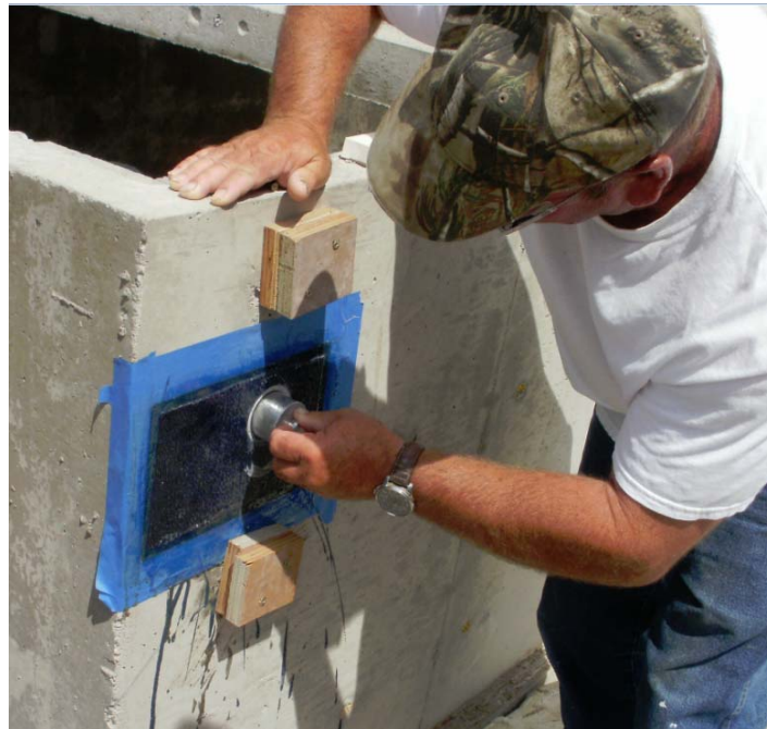
Figure 23B – Dolly Installation for ASTM D7522 Testing
