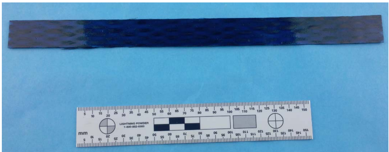
Figure A18 – \frac{3}{4} " Wide by Ten Inch Long Coupon for ASTM D3039 Test
