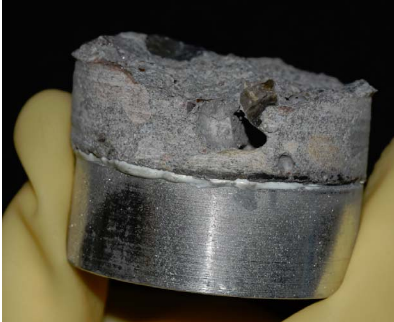
Figure A6 – Patti Micro Dolly and Concrete Failure Mode G
