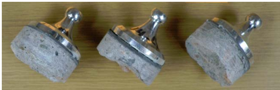
Figure A9 – DeFelsko Dolly and Concrete Failure Mode G
