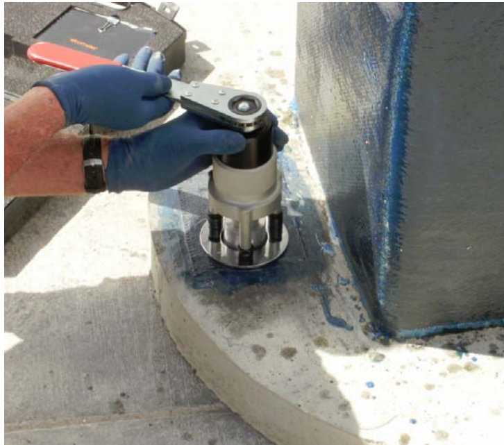
Figure 25B – Installation of the Loading Fixture for ASTM D7522 Test
