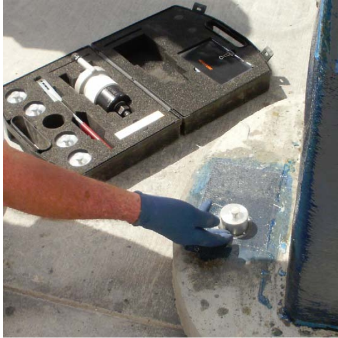
Figure 24B – Preparing to Perform ASTM D7522 Post-Installation Testing
