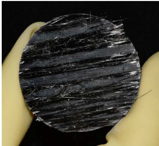
Figure A7 – Patti Micro Dolly and Through Fiber Failure - Mode B
