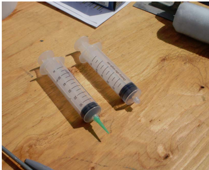
Figure 21B – Syringe for Injecting Void Pocket with Saturant
