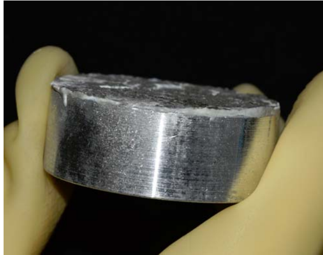
Figure A8 – Patti Micro Dolly and Failure at Plasite to Concrete Interface - Mode A
