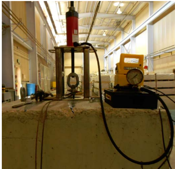
Figure A12 – Tensile Testing of FRP Anchor at LANL
