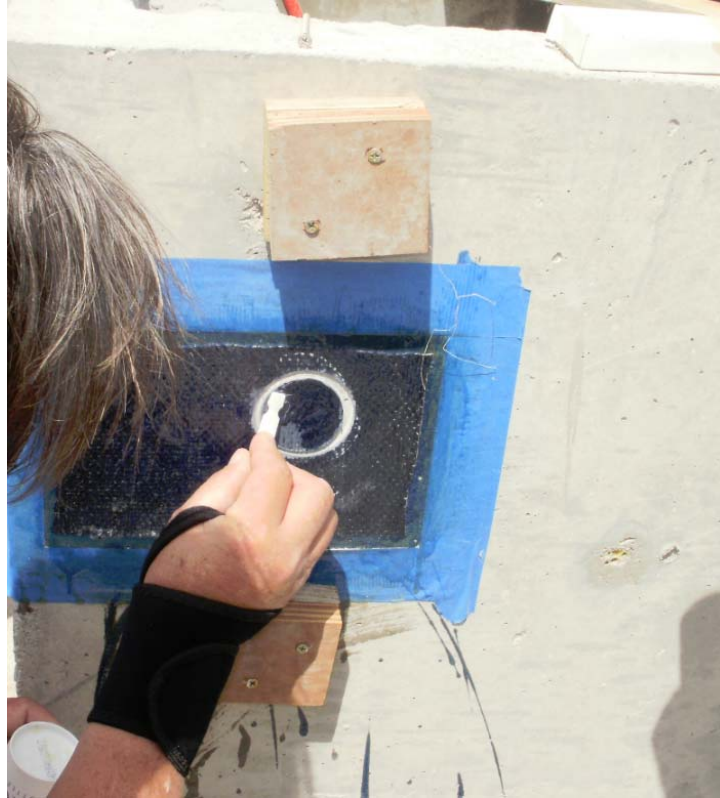
Figure 22B – Preparing a Cored FRP Sample for ASTM D7522 Testing
