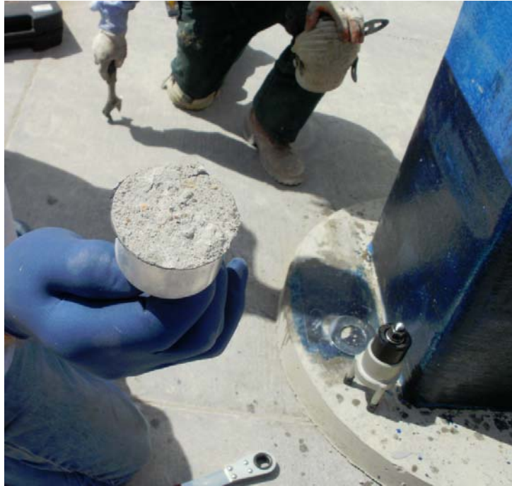
Figure 26B – Dolly Following Failure
