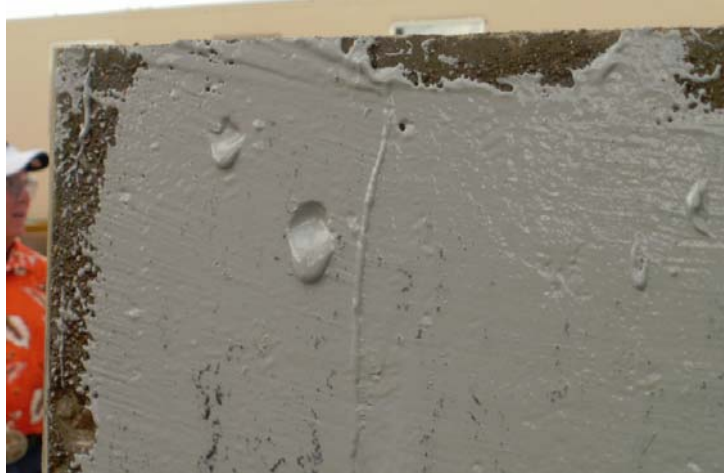
Figure 8B – Oozing of Putty
