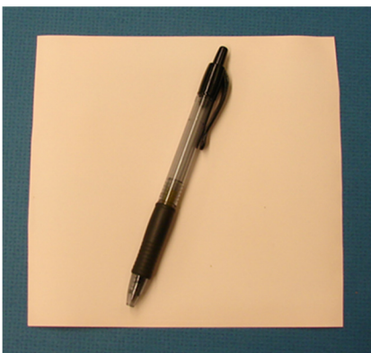
Figure V- 219: Composite membrane of 50vol.% Ohara glass ceramic powder and PEO+ LiTf salt (on blue background)
