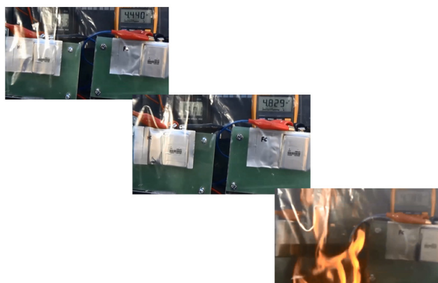
Figure V- 274: Overcharge testing on NMC111/graphite cells filled with hydrocarbon (left) and Daikin fluorinated electrolyte (right)
