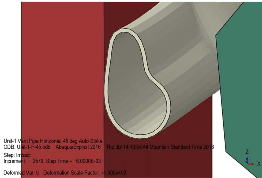
Figure 4 – Simulation of Impact of Pipe and Back Wall, with Missile Rebound
