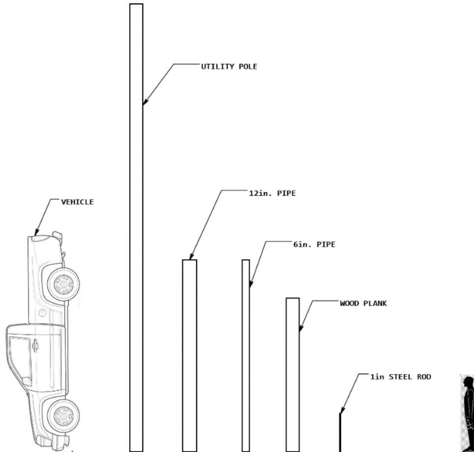
Figure 1 – The Six Common Tornado Missiles
