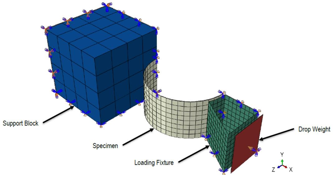
Figure 2 - Finite Element Model to Simulate Experimental Pipe Impact Tests
