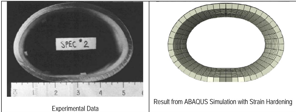
Figure 3 - Benchmark of Finite Element Model against Experimental Pipe Impact Data
