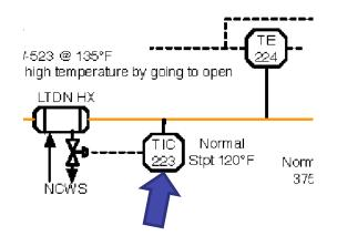
Controller temperature sensor on letdown line fails low
