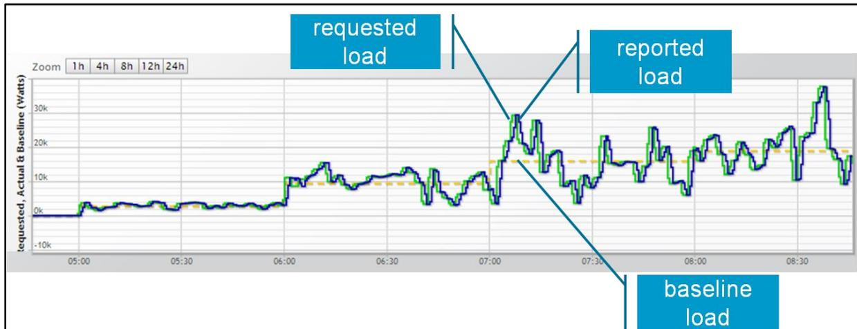
**Figure 10. Near Coincidence of Requested vs. Reported Load from GETS System Aggregated Group in Response to Simulated ACE Signals for Frequency Regulation**
