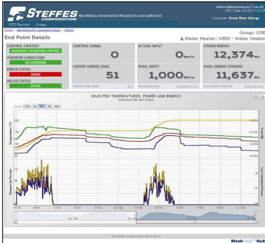
Figure 8. Steffes Data on Temperature, Power, and Energy for an Individual Water Heater
