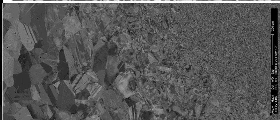
Alloy C22, solution strengthened corrosion resistance
