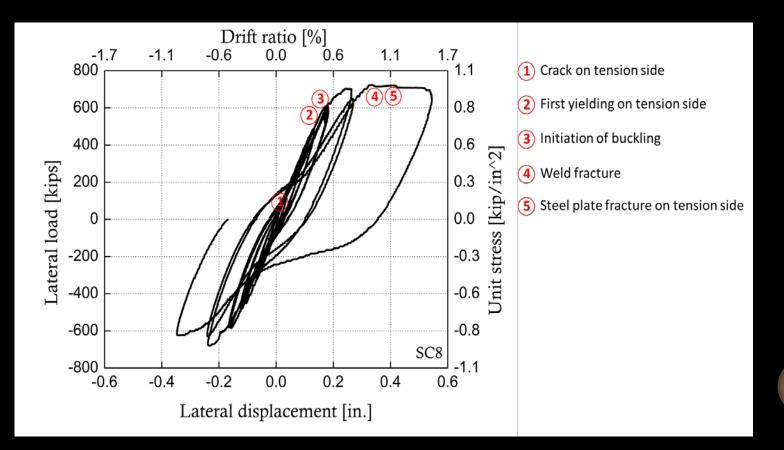
SC-Wall Pier Specimens: Cyclic In-plane Shear at Ambient Condition – Experimental Observations
