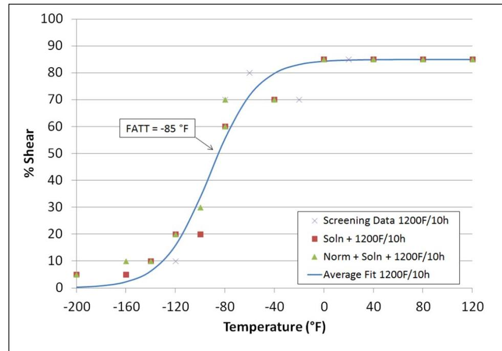
Solution Annealed at 2050F/10hrs, quenched, normalized 1650F and tempered at 1200F/10 hrs
