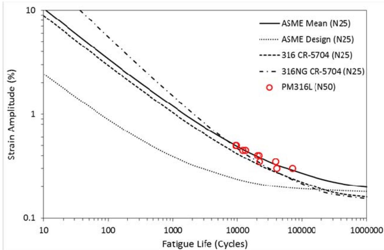
Measured 316LSS LCF data compared with ASME and NUREG- 5704 data.
