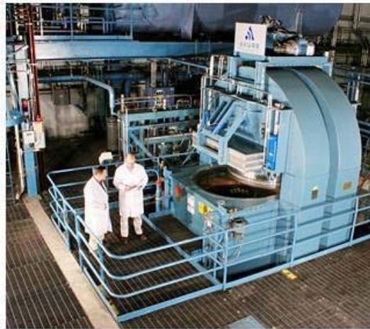
3. Hot Isostatic Pressing Apply High Pressure (>15,000psi), Temperature (>2000F)
