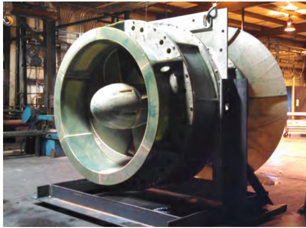
Figure 1-9. Composite housing with combined turbine/generator assembly
