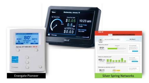
Study results obtained from the testing period, June 1 through Sept 30 of 2010, show that the initial hypothesis of 1.3 kW of max demand reduction is achievable. In particular the VPP/PCT combination provided the greatest amount of demand reduction, approximately 1.96kW or 58%, for the average VPP/PCT participant when compared to the control group. This result is likely explained by the automated response of the thermostat, which is lacking in the web and IHD treatments.
