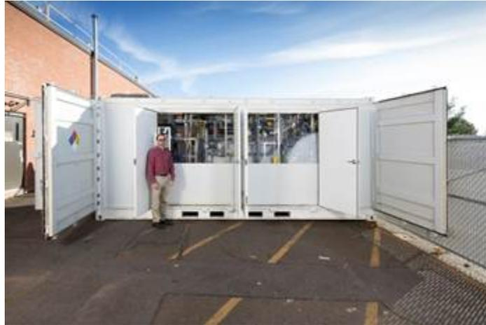
Figure 17: Vanadium redox flow battery [13].
