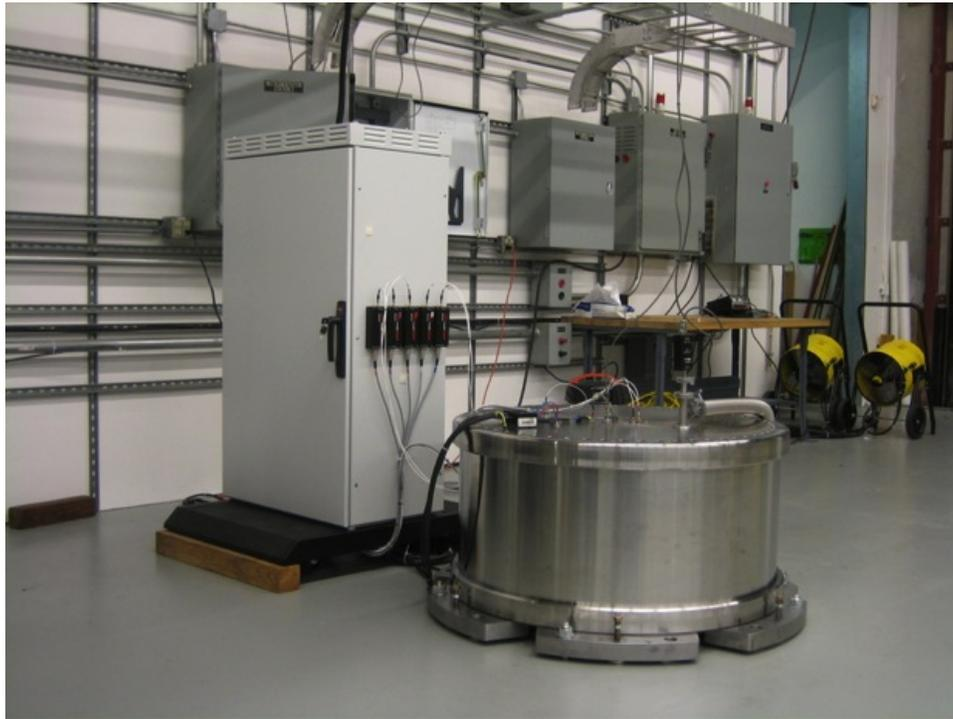
Figure 14: Amber Kinetics, first generation flywheel system [11].
