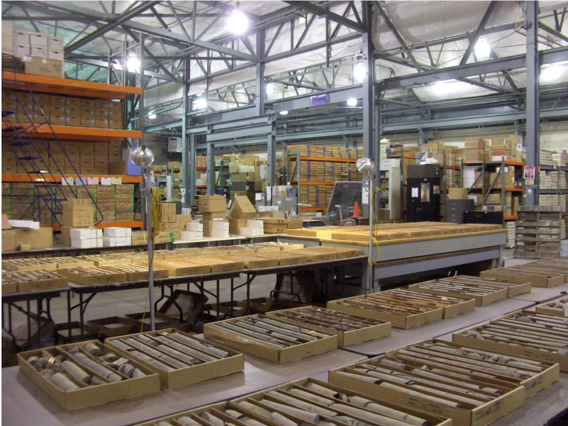
Figure 7. Core layout area and storage at the EGI Sample Library. The core in the foreground is part of an extensive collection from the Medicine Lake geothermal field, California.
